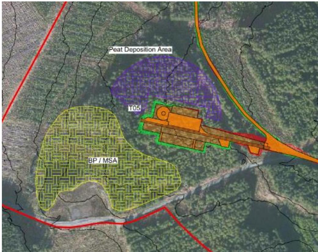
**Figure 9-22: Example of Peat Deposition and Borrow Pit / Material Storage Areas (BP/ MSA) near T5**
