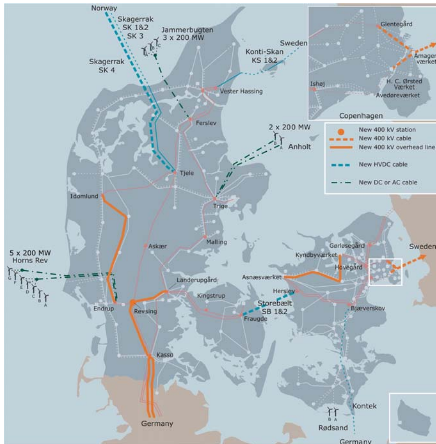
Figure 6 Expansion principle E – new 400 kV overhead lines on lower towers in a new design.
