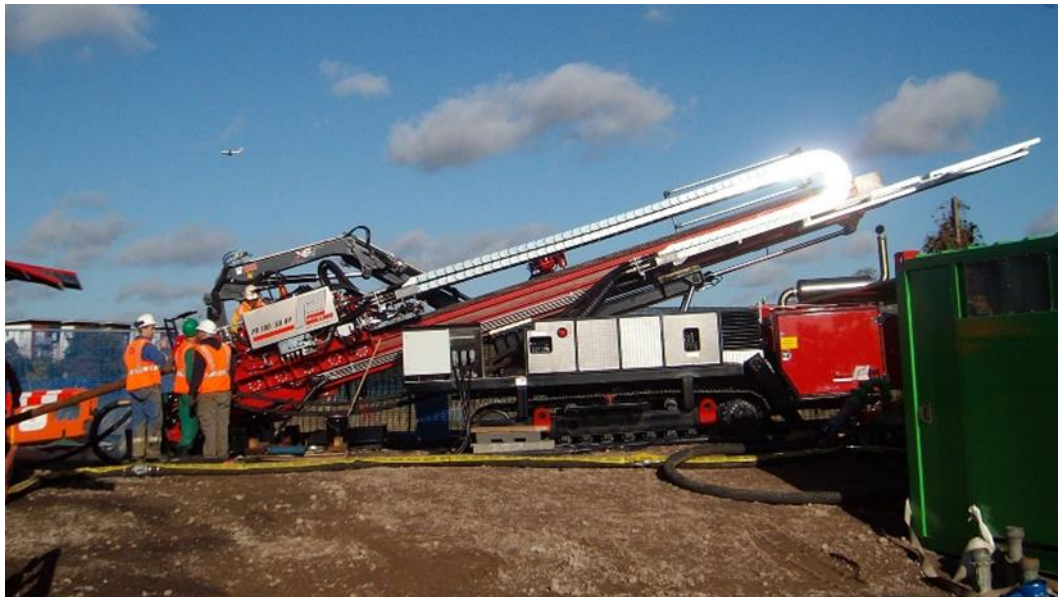
Figure 7: Photo of Typical Horizontal Directional Drilling Rig
