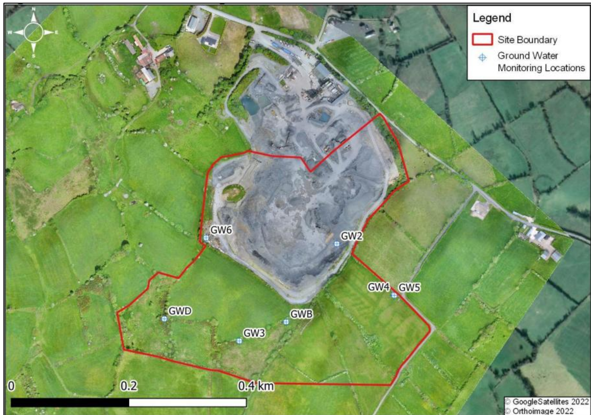
Figure 1. Groundwater Sampling Locations as per EIAR (Source MOR Environmental)
