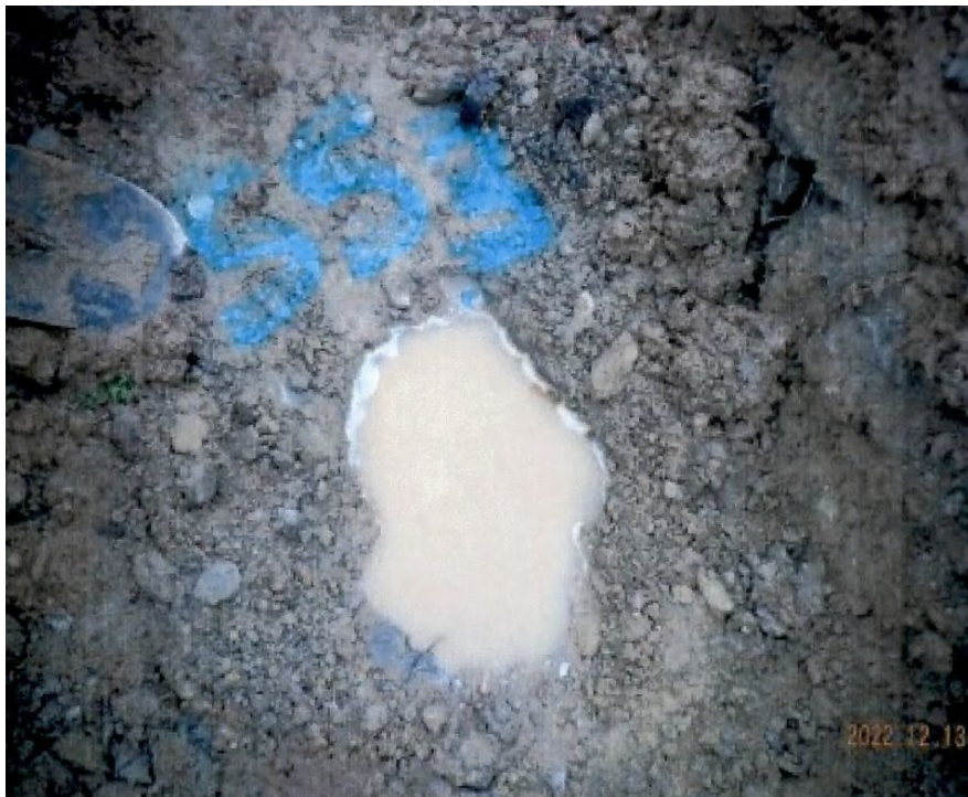
Figure 2.5 Photograph of the subsurface percolation test hole SS3 carried out in the imported infill material
