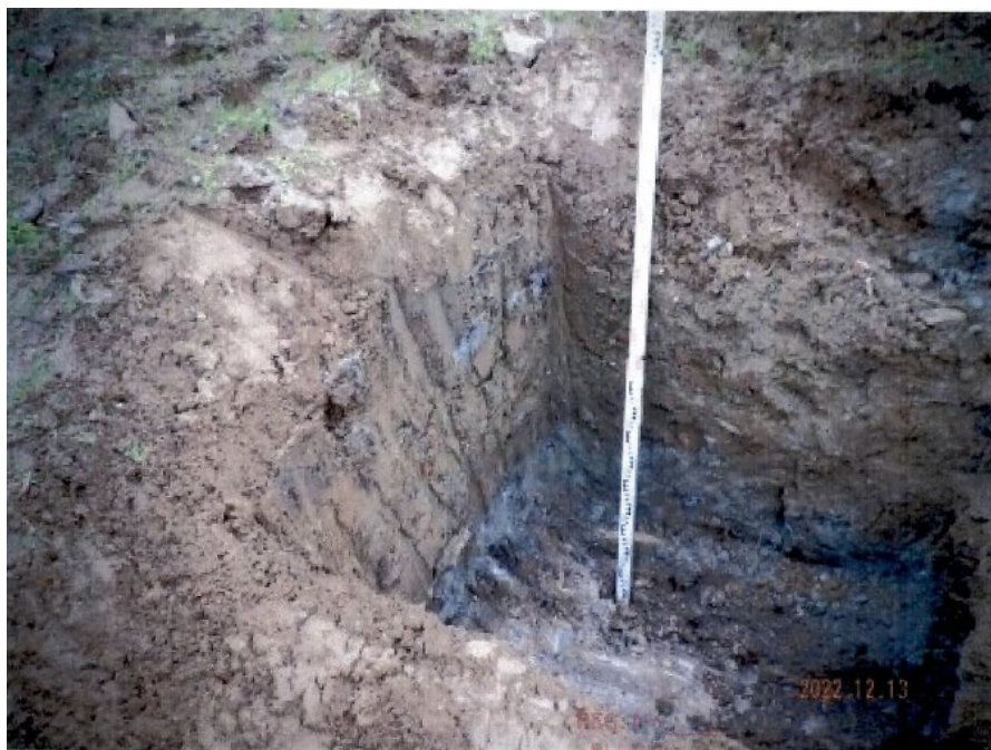
Figure 2.2 Photograph of the trial hole with evidence of the existing ground and imported material
