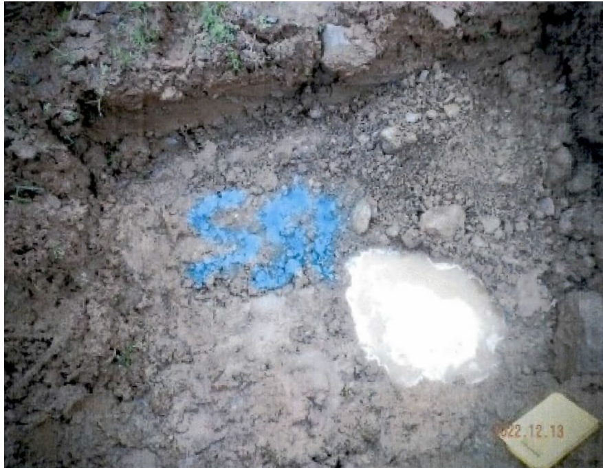
Figure 2.4 Photograph of the subsurface percolation test hole SS2 carried out in the imported infill material
