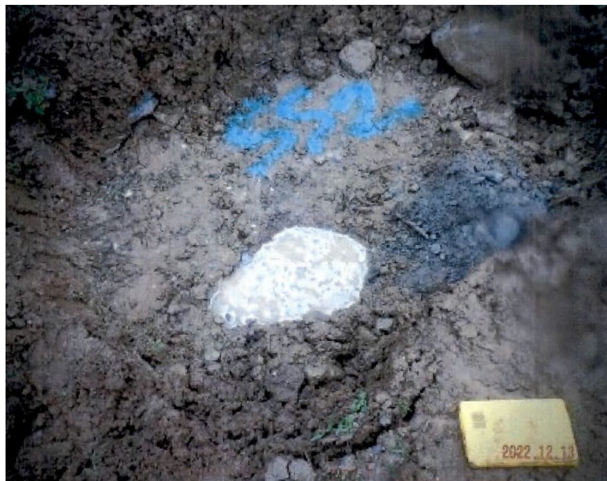
Figure 2.4 Photograph of the subsurface percolation test hole SS2 carried out in the imported infill material
