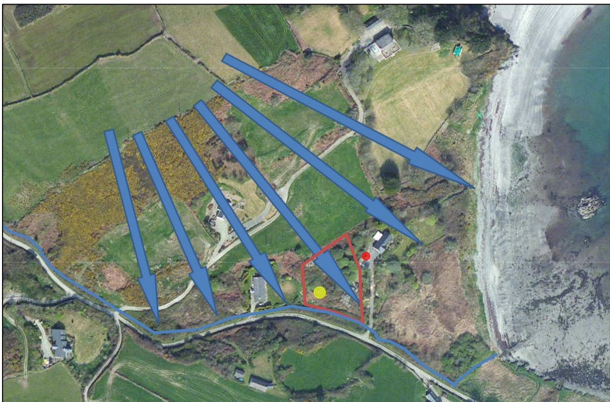
Figure 2.6 Groundwater flow direction and approx. location of neighbouring well (red) and proposed WWTP (yellow)
