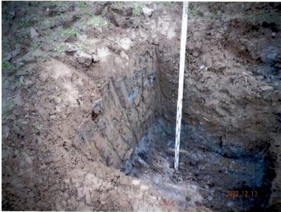
Figure 2.2 Photograph of the trial hole with evidence of the existing ground and imported material
