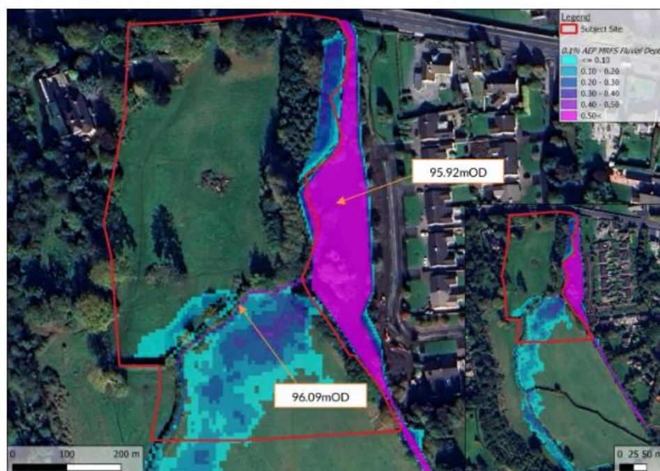
Figure 4-4 Predicted Flood Depths at Existing Site [1,000-year MRFS]
