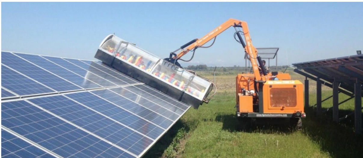
Figure 14 – Solar farm cleaning equipment
