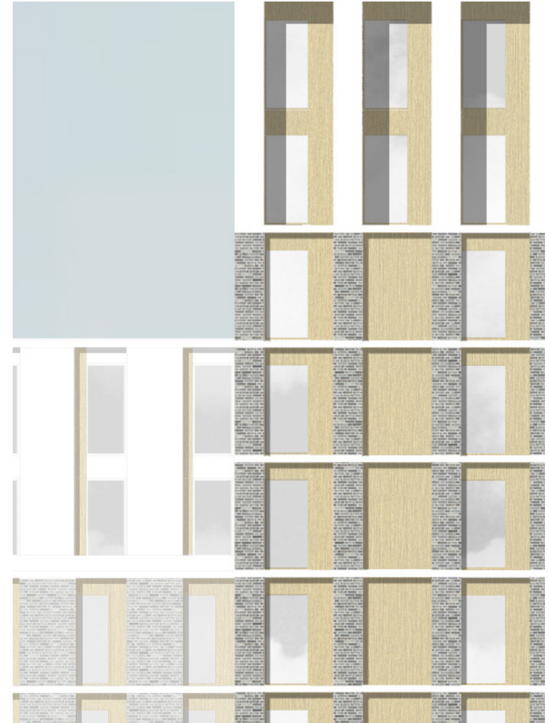
Horizontal precast capping with overhang minimising water flow down facade flashed with aluminium window to avoid staining from birds ect...
