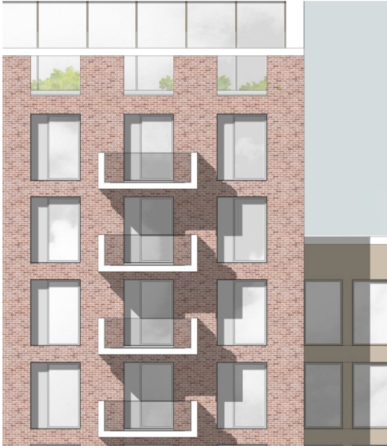
Prefabricated balcony 'bucket', to ensure design quality and consistency through scheme.
