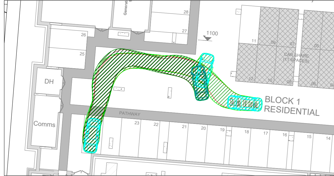
2.) PARKING SPACE 24 ACCESS (BLOCK 1) SCALE 1:250
