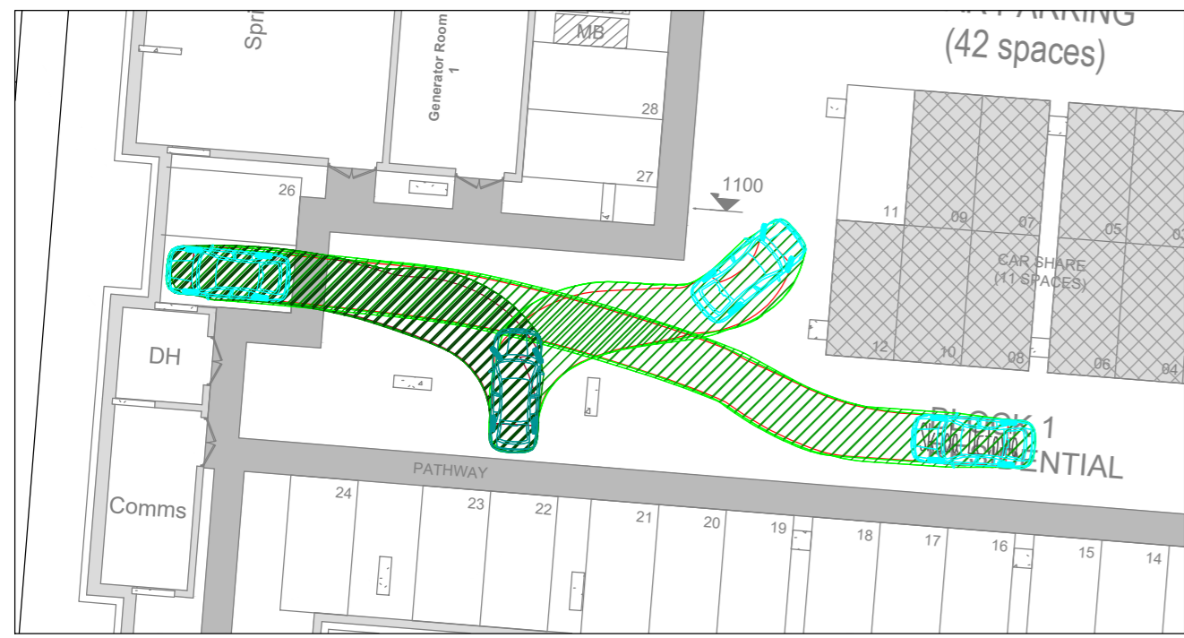
1.) PARKING SPACE 25 ACCESS (BLOCK 1) SCALE 1:250
