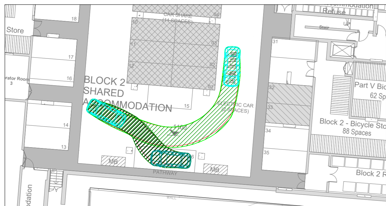
7.) PARKING SPACE 36 ACCESS (BLOCK 2) SCALE 1:250
