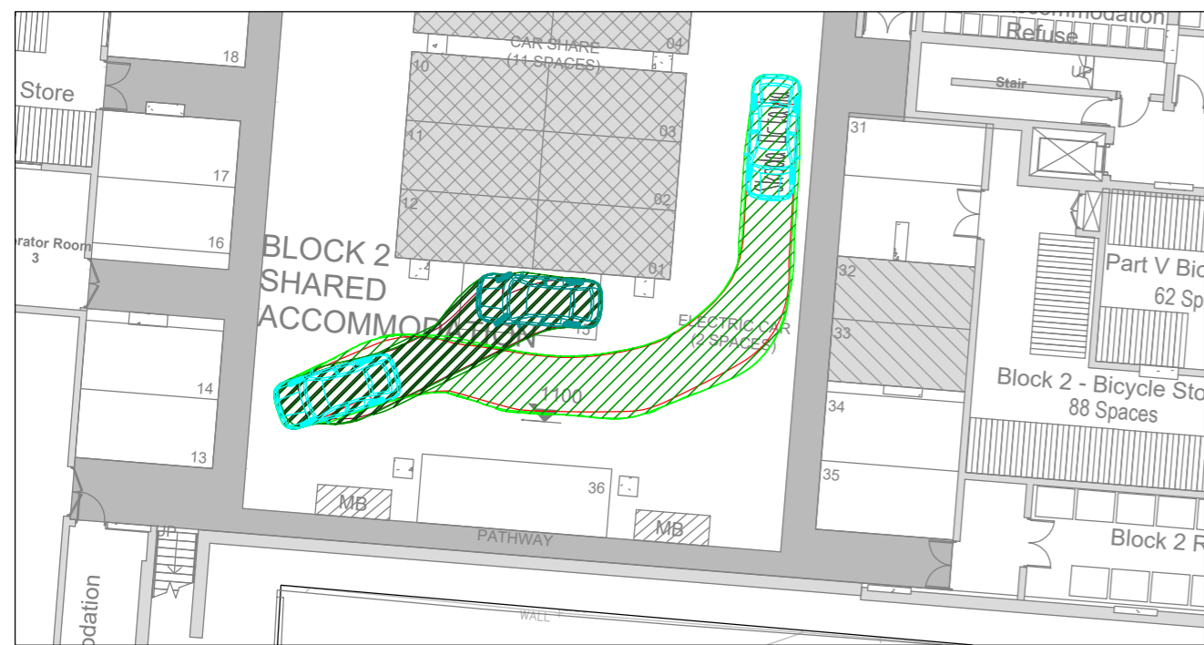
8.) PARKING SPACE 15 ACCESS (BLOCK 2) SCALE 1:250
