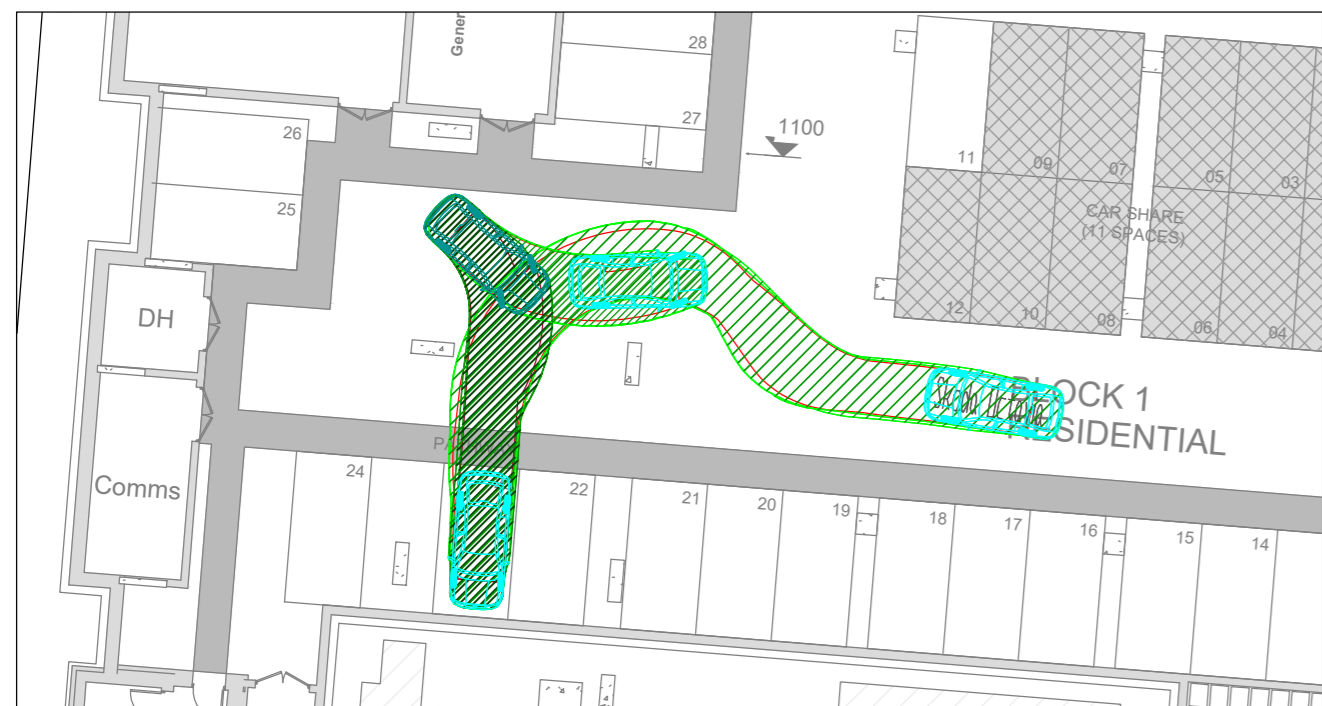
3.) PARKING SPACE 23 ACCESS (BLOCK 1) SCALE 1:250
