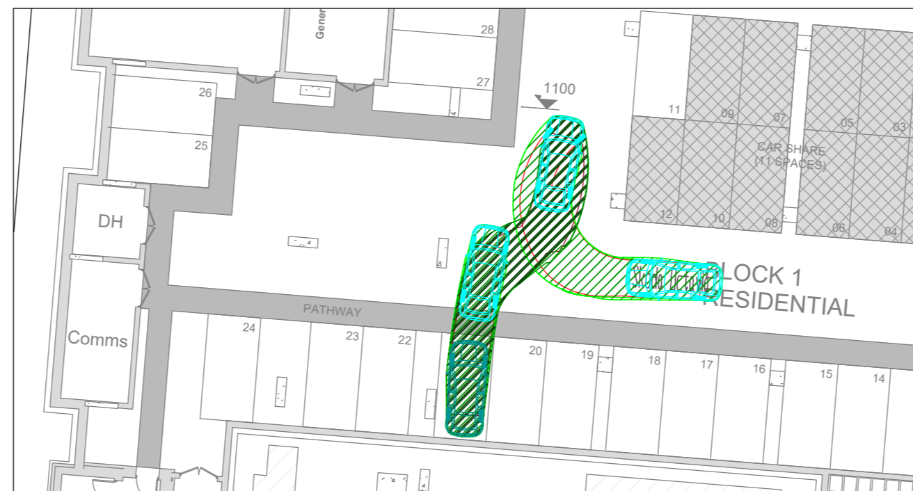
5.) PARKING SPACE 21 ACCESS (BLOCK 1) SCALE 1:250
