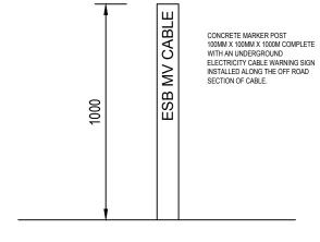
Marker Post and Marker Plate Details Scale 1;5
