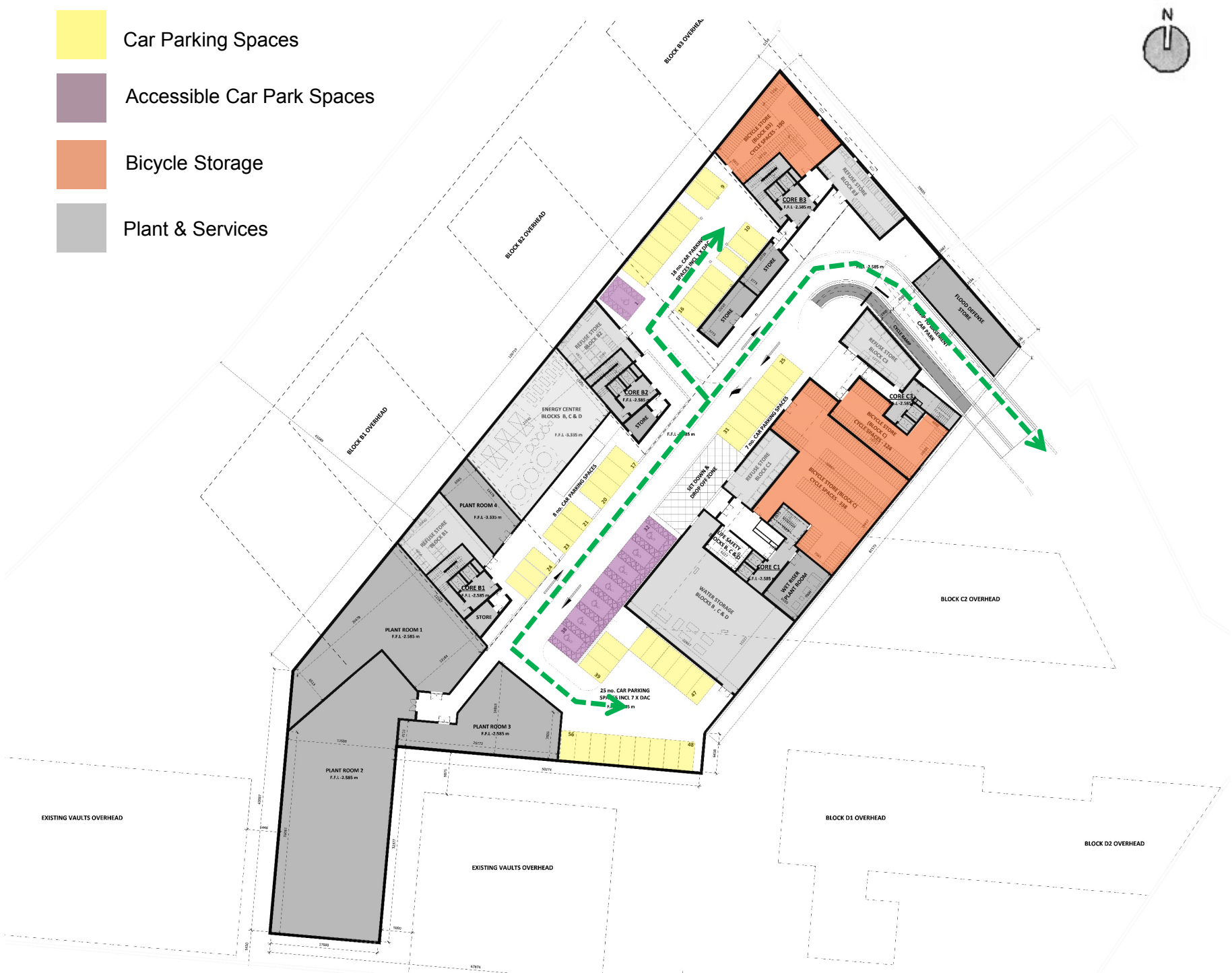
Basement Access Plan
