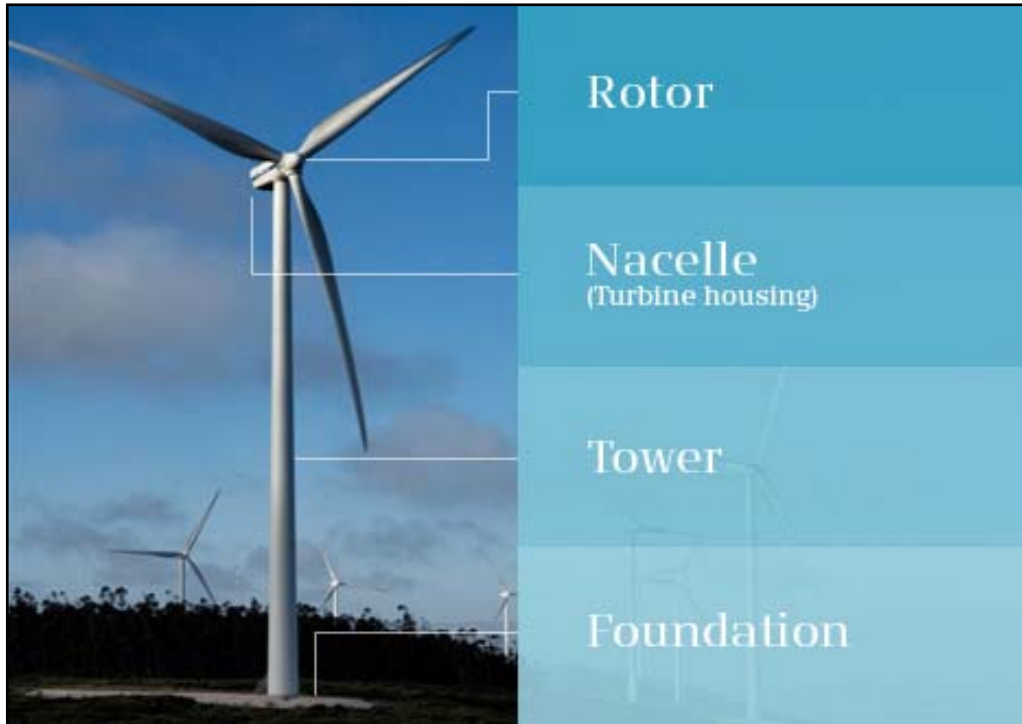
Plate 4-1 Wind Turbine Components.
