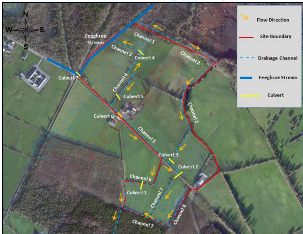
Figure 10.2: Existing site drainage network
