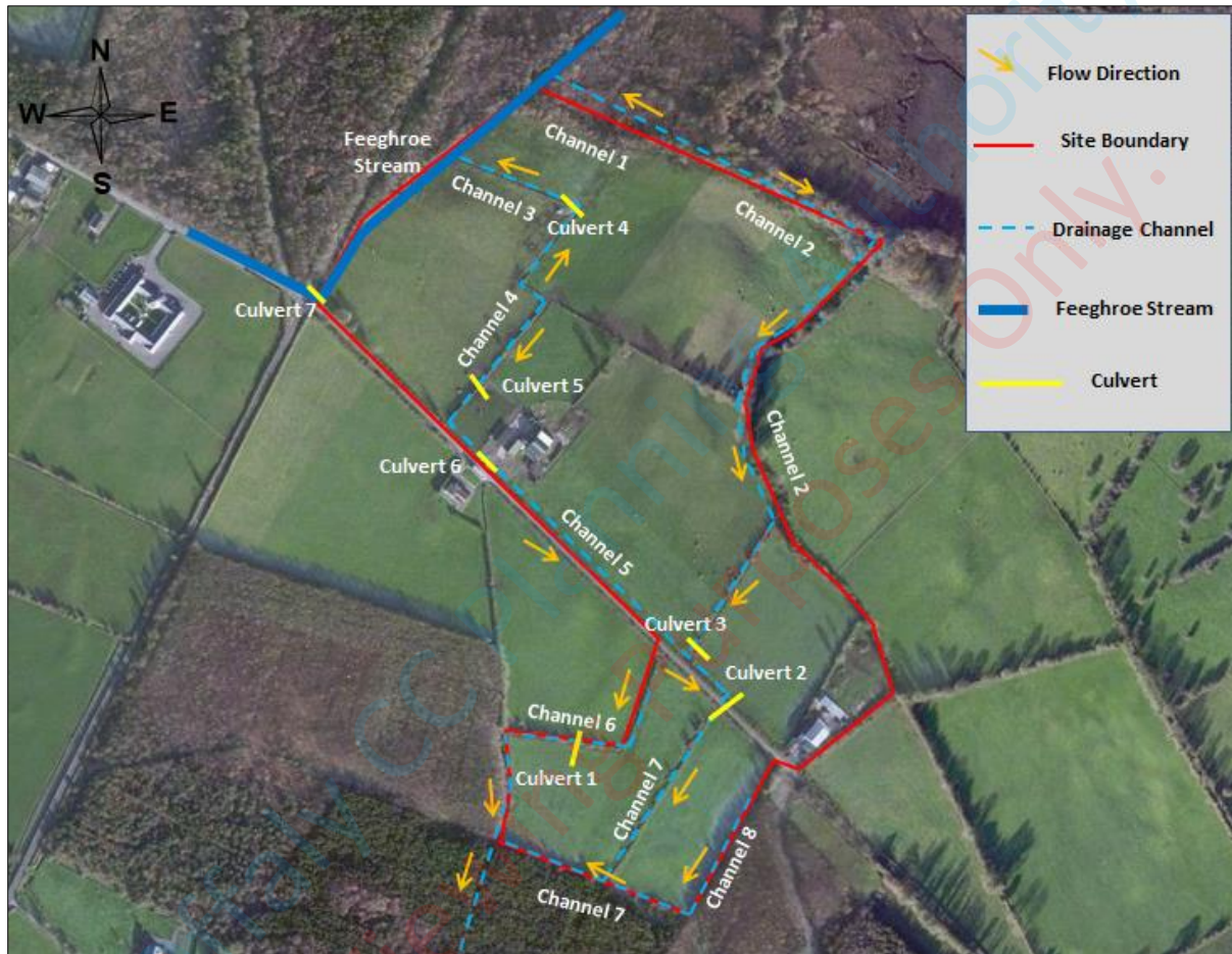
Figure 11.3: Site hydrology showing the drainage channels, culverts, flow directions and Feeghroe Stream.
