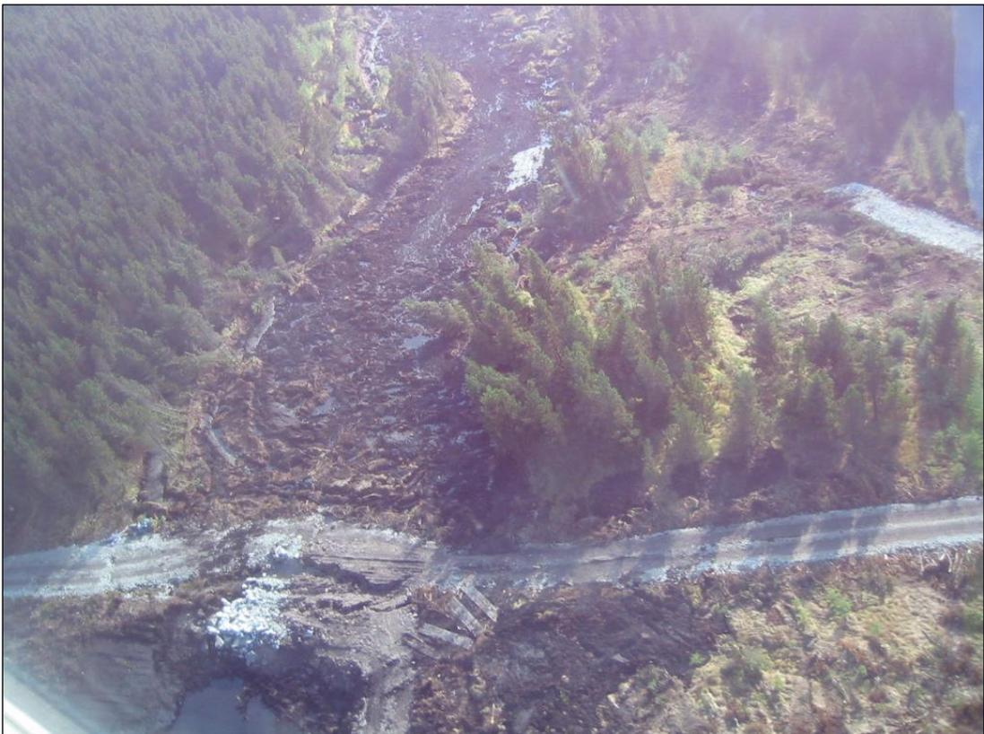
**Plate 16-2 – Aerial view of the head of the slide at Turbine T68 (October 2003)**
