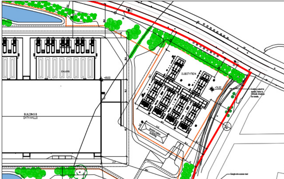
Figure 3.1 Permitted AIS Substation in north-east corner of Permitted Development site (shaded cream)
