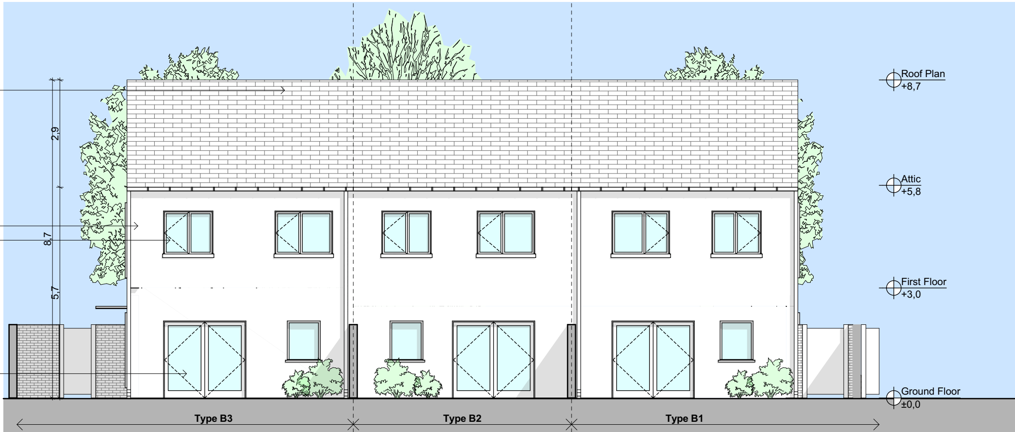
Rear Elevation SCALE 1:100
