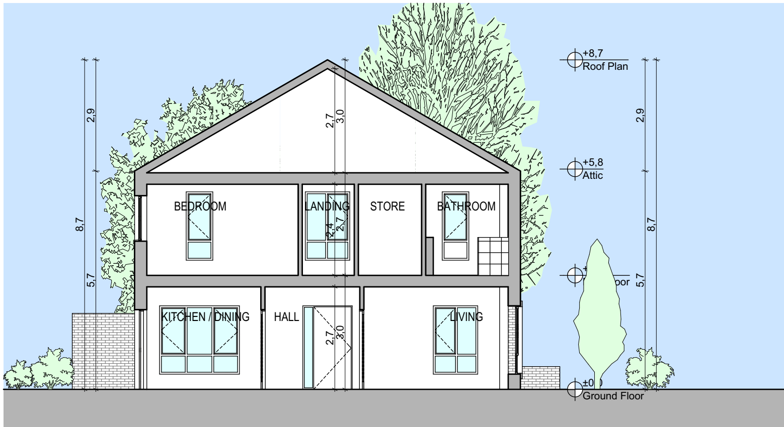
Typical Building Section through B3 - Section 2 SCALE 1:100
