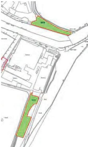
**Figure 10.3: Site Compounds** (extracted from Drawing No 1065 and in Chapter 5). Site Compound 5 (SC5) located at North Pier, SC6 located at South Beach. Do not scale
