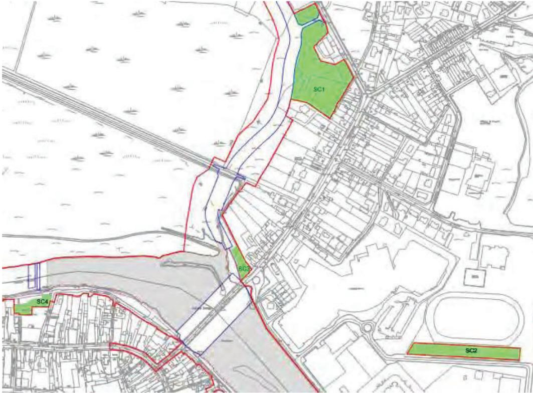
**Figure 10.2: Site Compounds** (extracted from Drawing No 1065 as described in Chapter 5). Site Compound 1 (SC1) located in Arklow Marsh, SC3 located on north bank (Ferrybank), SC2 located to the east near running track, SC4 located at Main St carpark on south bank near Riverwalk. Do not scale
