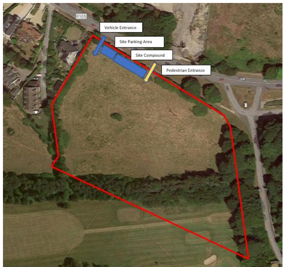
Figure 5 – Initial Site Set Up with Compound (Site Red Line Boundary Indicate only)
