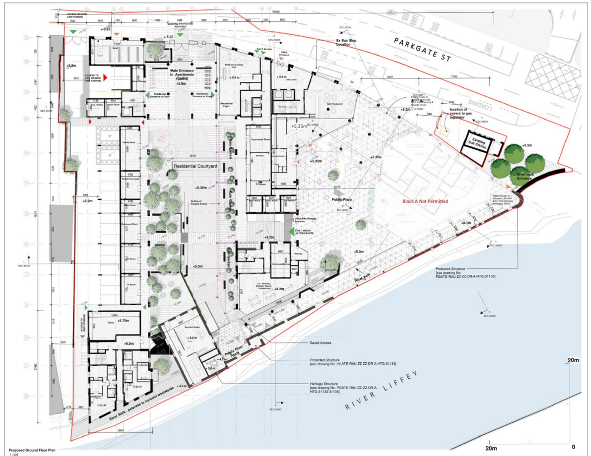
Figure 3.5: Extract from drawing PGATE-RAU-ZZ-00-DR-A-GAP-31100 - Ground Floor Plan, prepared by Reddy Architecture + Urbanism, showing ground floor area of consented and refused development under ABP-306569-20
