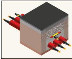
The circuit between the connection point and the converter station can be an underground cable, if they are located within a number of kilometres of each other. Otherwise, the circuit will be an overhead line. As an underground cable, the circuit would be installed in ducts under the road network, which would be fully re-instated.
