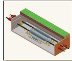
This is where the land circuit will connect to the submarine circuit by way of an underground transition joint. This will be installed behind the beach where the submarine circuit comes ashore. The landfall point will be fully re-instated following completion of the works.
