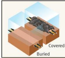
The submarine circuit between Ireland and France will be approximately 500 km. It will be either buried beneath the seabed or laid on the seabed and covered for protection.
