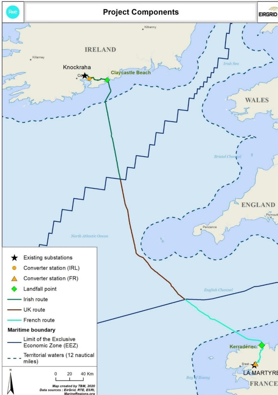
**Figure 2.2: Overview of the Entire Route of the overall Celtic Interconnector project (Source: TBM Consulting Group)**
