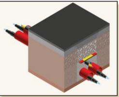
The circuit between the converter station and the landfall point will be by underground cable installed in ducts under the road network, which will be fully re-instated. The total length of this circuit is expected to be between 30 – 40 km.
