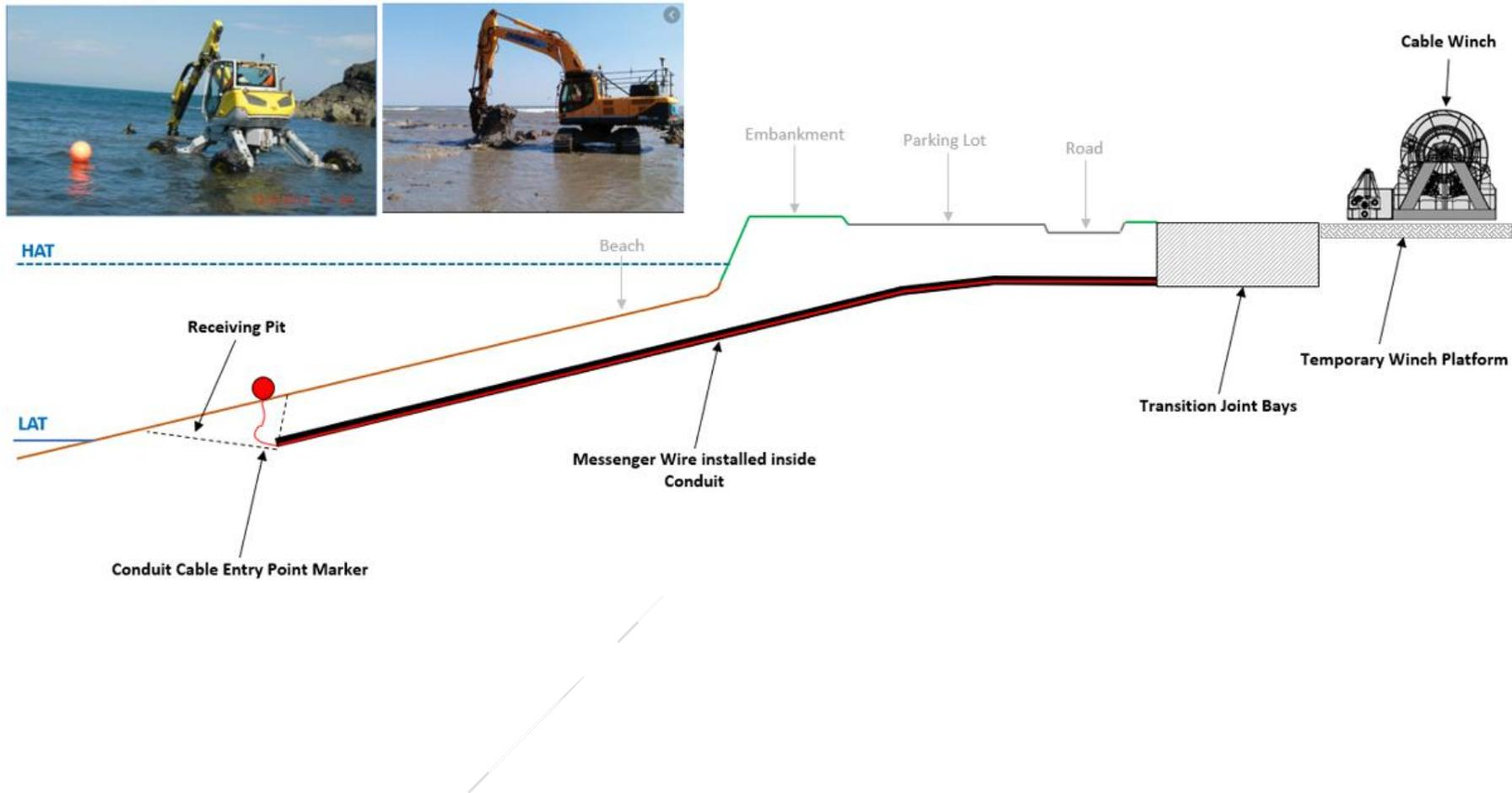
The submarine cables shall arrive on site aboard a cable lay vessel. The messenger wire shall be transferred to the cable lay vessel for connection to the end of the submarine cable as shown in Figure 5.11.
