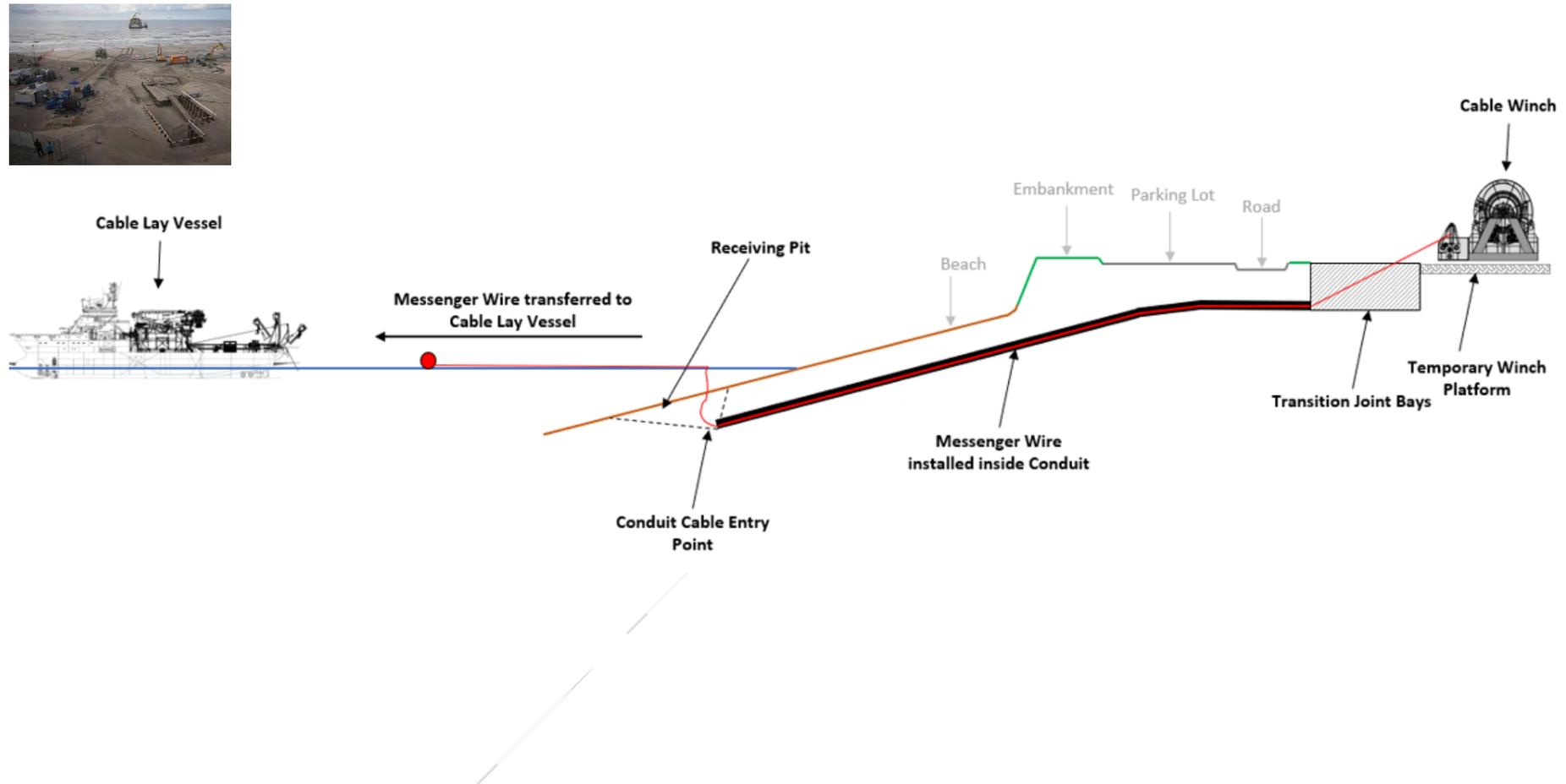
Figure 5.12 Submarine Cable floated to Shore
