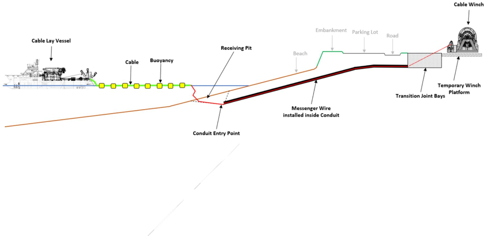
Figure 5.13 Phase Two Post-Construction
