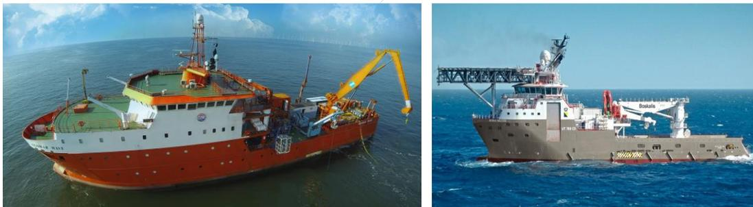
The cable lay vessel (approx. 90 POB) shall arrive at site fully laden with all equipment required to perform the installation activity. The method to transfer the plough from the vessel to the beach may require an additional abnormal load movement through Cork Port. However, it is envisaged that the plough shall be transferred on a shallow draft barge at high water and lifted by an on-board crane and placed in the receiving pit.
