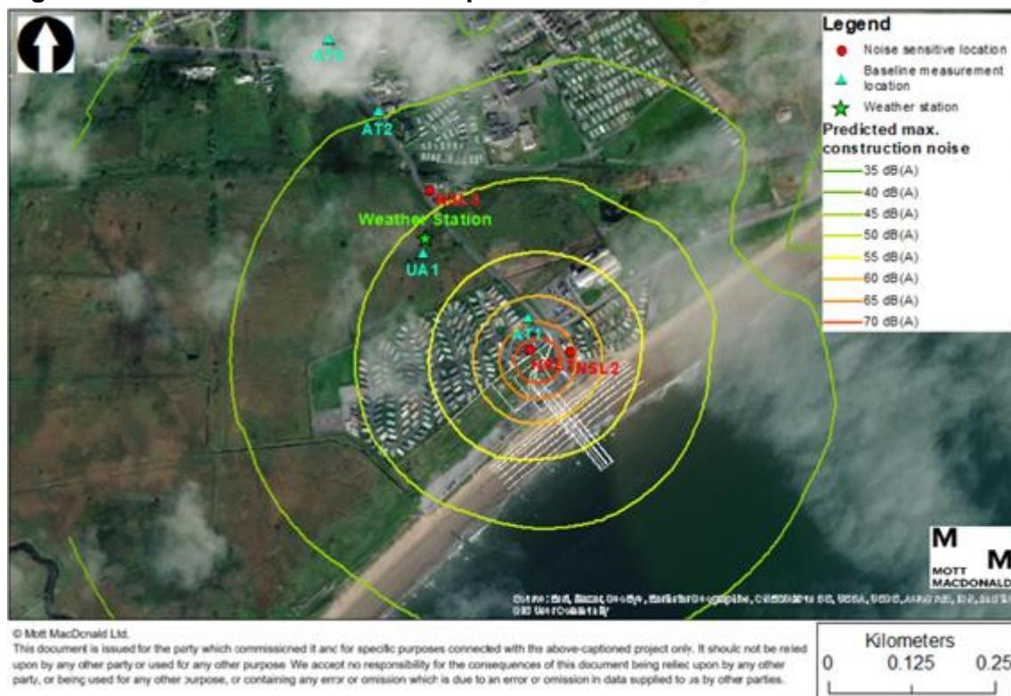
The sound source level from sheet piling within 6m from the source if used for the installation of a cofferdam at high tide is predicted to not exceed a worst case of 84dB(A) in line with published data (Subacoustech, 2018; Paulus et al, 2008). The source level of land is
