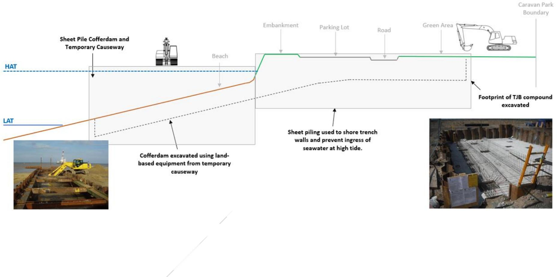
Figure 5.7 Temporary Works – Conduit installation
