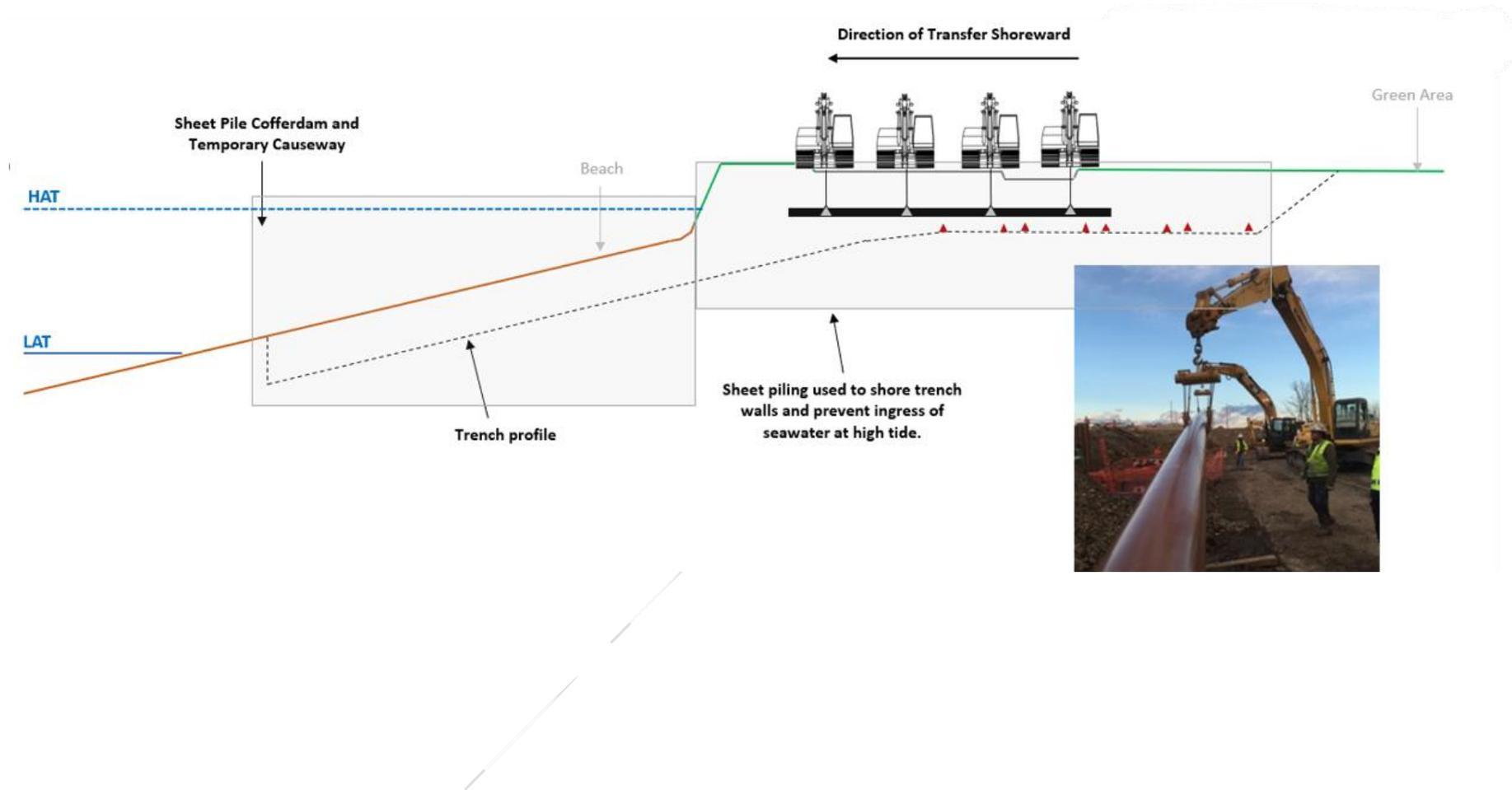
Following the installation of the conduits any temporary conduit supports within the trench will be removed and a messenger wire will be pre-installed within the conduits. The trench spoil will be returned to the trench to re-instate the beach to its prior condition. The temporary causeway and cofferdam will be removed and the car park will be re-instated.
