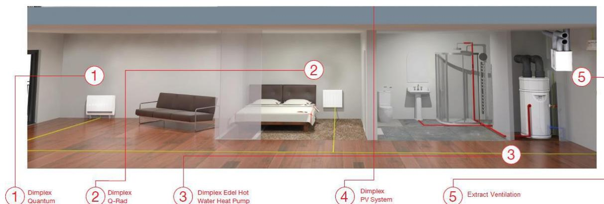
Figure 5 – Typical Air-Source Heat Pump with electric panel heaters arrangement
