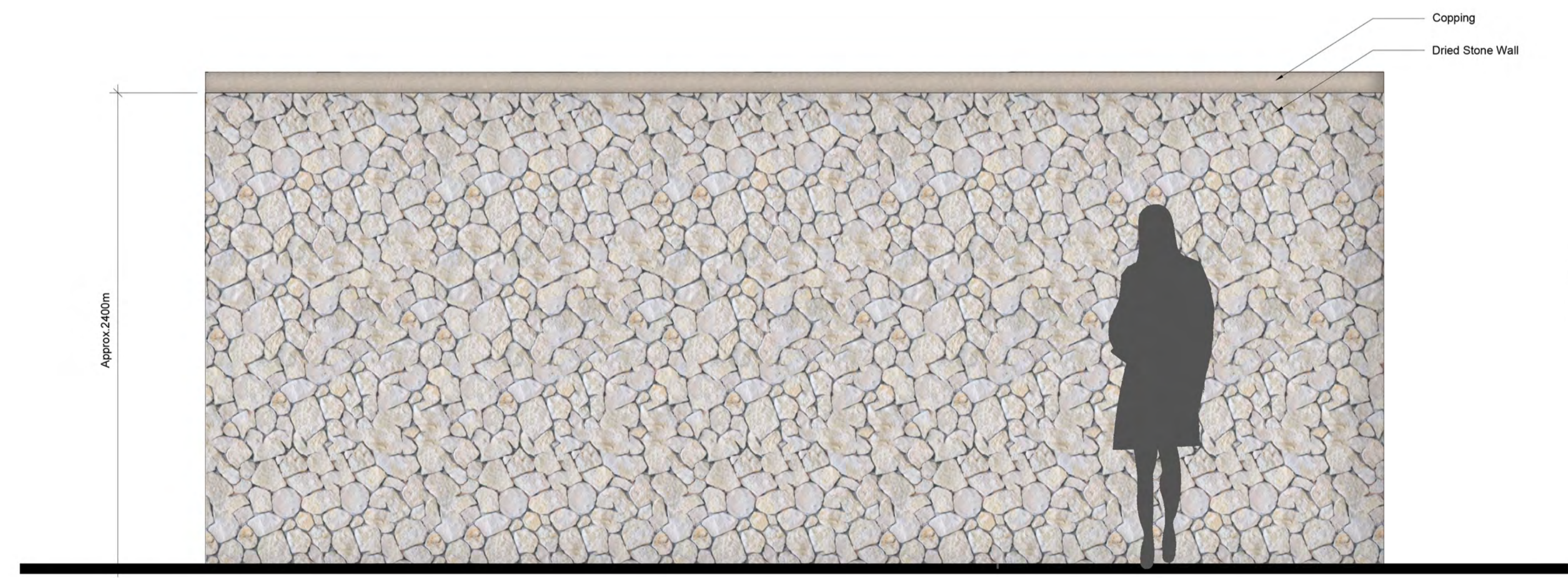
2 South Boundary: Proposed Stone wall scale 1:20 @A1
