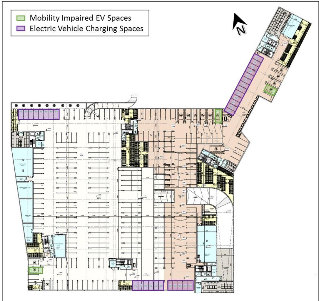
**Figure 4.16: Electric Vehicle Charging Spaces within Basement**
