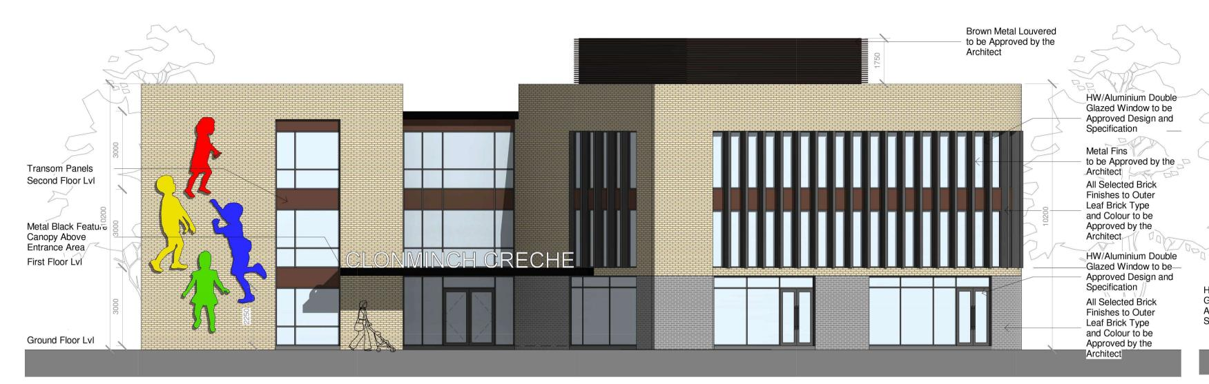
Brown Metal Louvered to be Approved by the Architect Metal Fins Metal Fins to be Approved by the Architect to be Approved by the Architect Transom Panels HW/Aluminium Double Glazed Window to be Approved Design and Specification All Selected Brick Finishes to Outer HW/Aluminium Double Leaf Brick Type Glazed Window to be and Colour to be Approved Design and Approved by the Specification Architect
