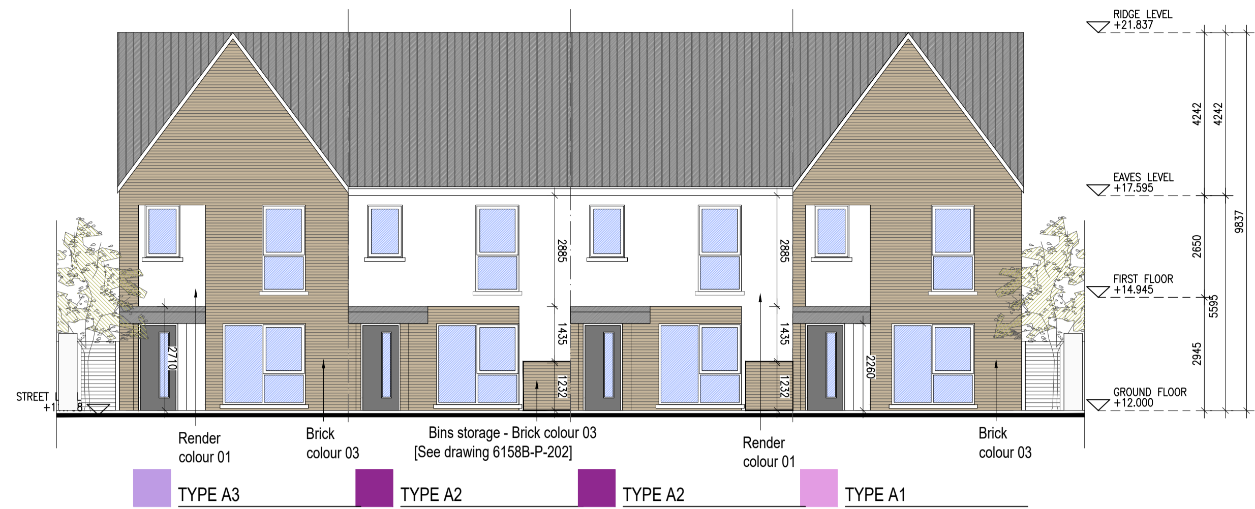
01 Type A1, A2, A3 - Front Elevations - Maynetown
