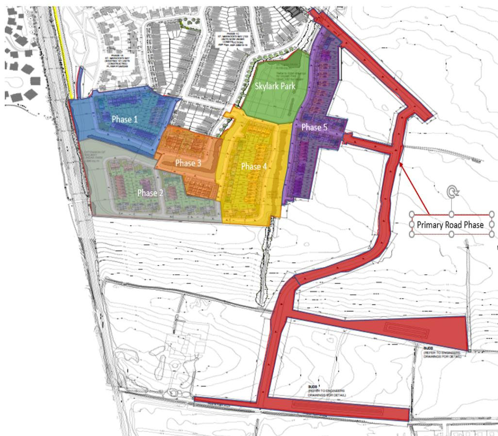
**Figure 3.4:** Indicative Site Construction Phasing Plan.
