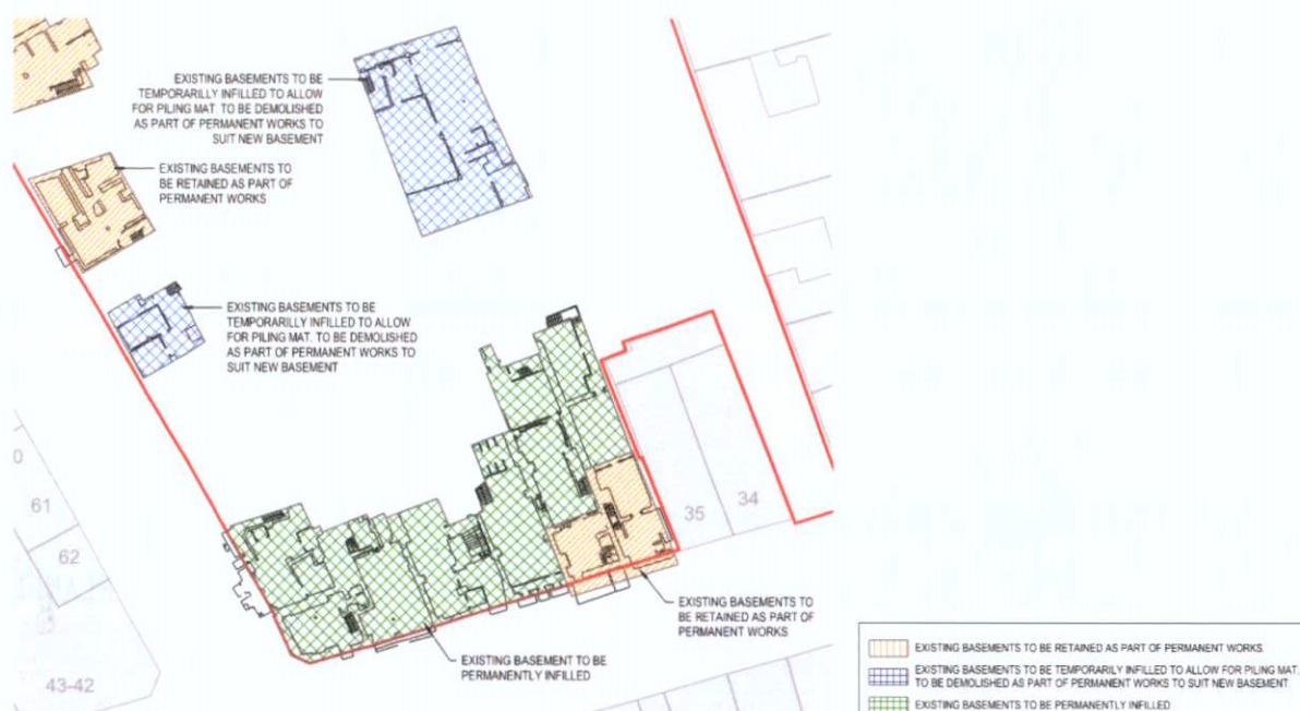
Figure 32 – Site 3 Existing Basements
