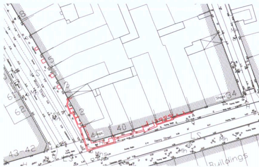
Figure 33 – Location of Existing Historical Pavement Vaults
