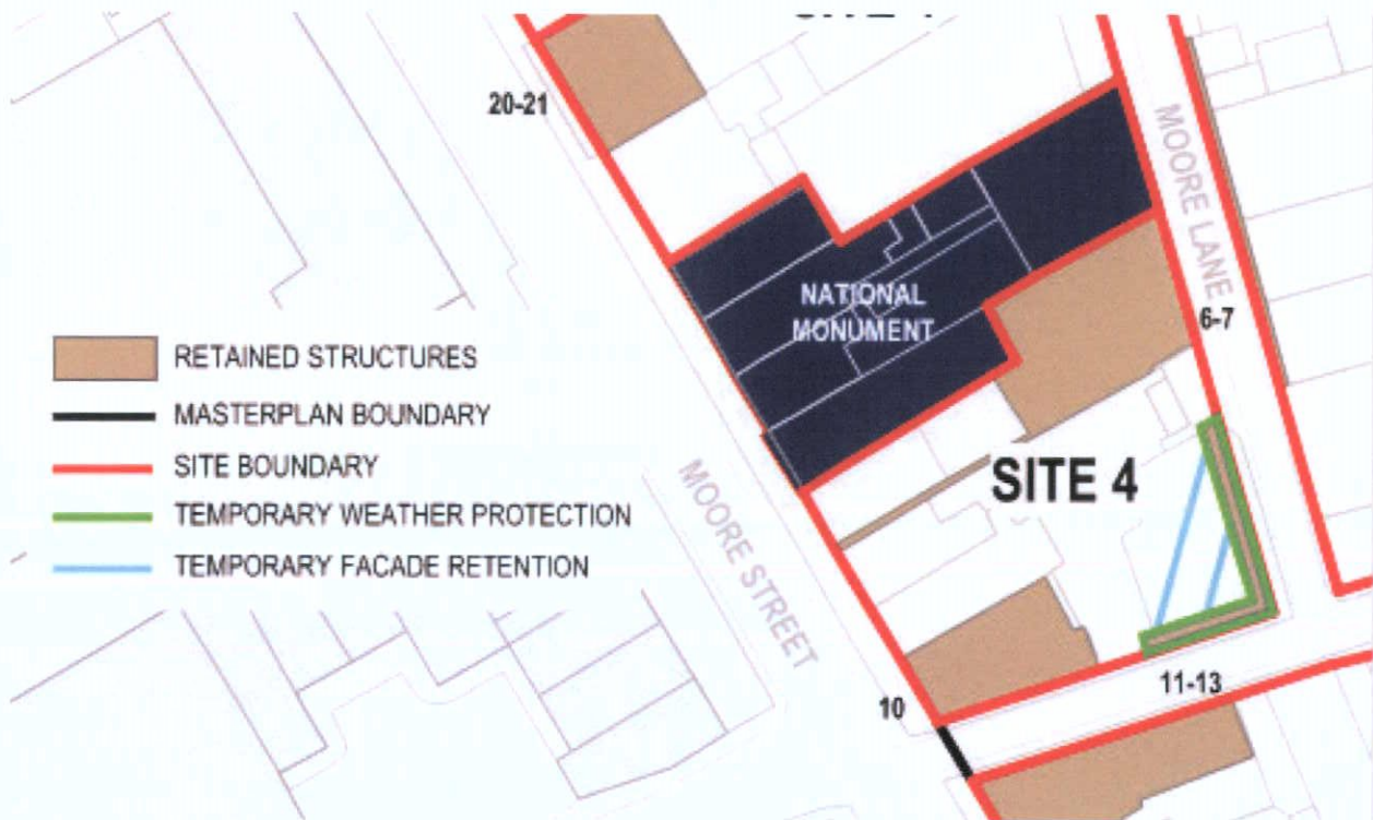
Figure 24 – Site 4 - Preliminary Temporary Works (5 Moore Lane)
