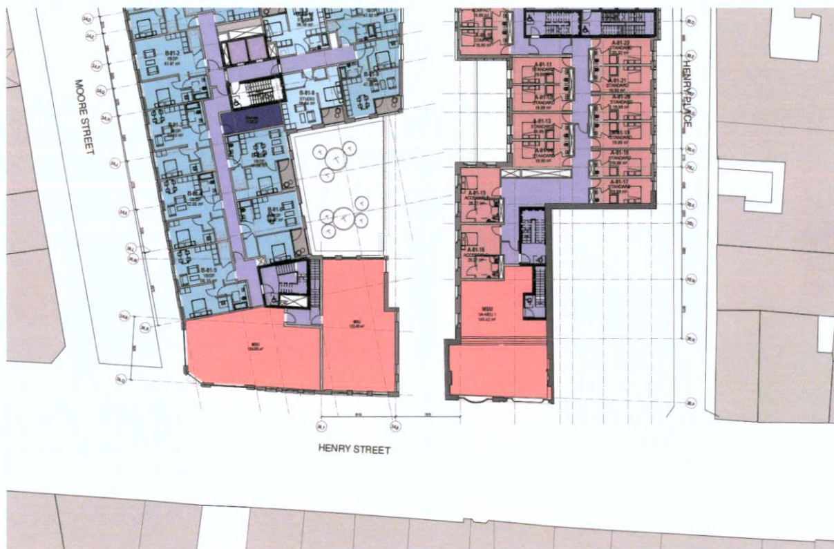
Figure 4.4: Extract from a First Floor Plan for 'Site 3' based on proposal c. February 2021 – Greater extent of No. 36 – 37 Henry Street retained as part of current 'Site 3' iteration.
