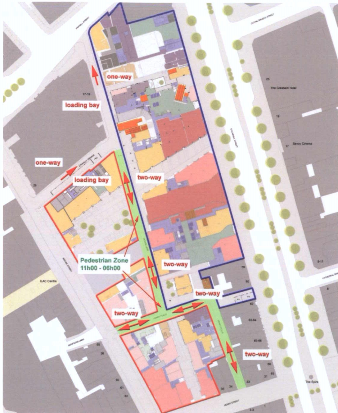
Figure 13.19: Street Layout – Proposed. Proposed Development outlined in red – future development outlined in blue.
