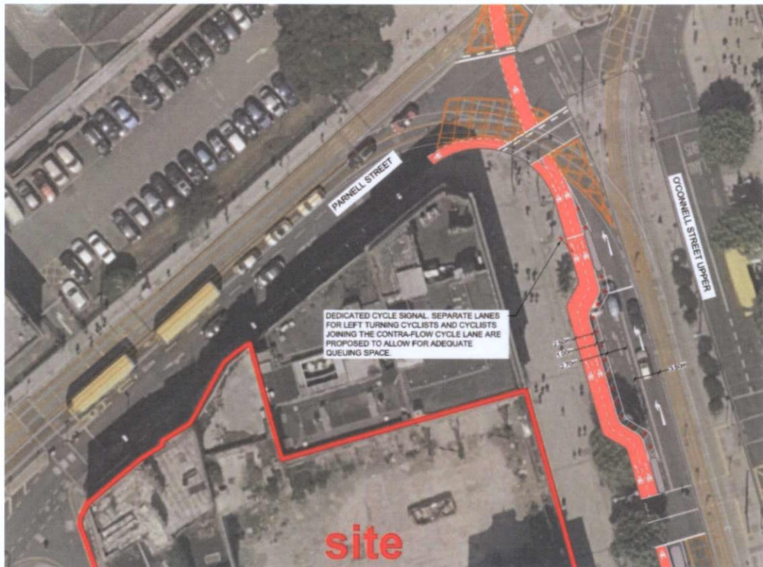
Figure 13.12: Parnell Square Contraflow Cycle Facility.
