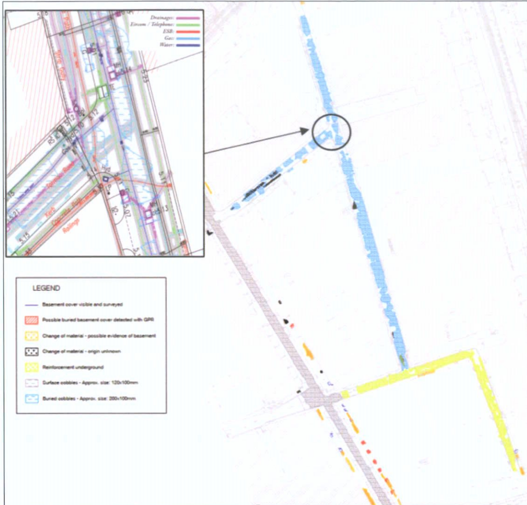
Figure 16.25: GPR survey of the lanes within the Dublin Central Masterplan area (inset shows the services with the lane).
