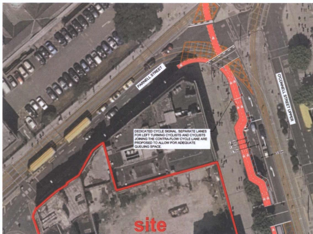
Figure 13.12: Parnell Square Contraflow Cycle Facility.
