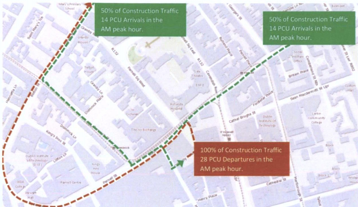
Figure 13.27: Construction Traffic Trip Distribution.
