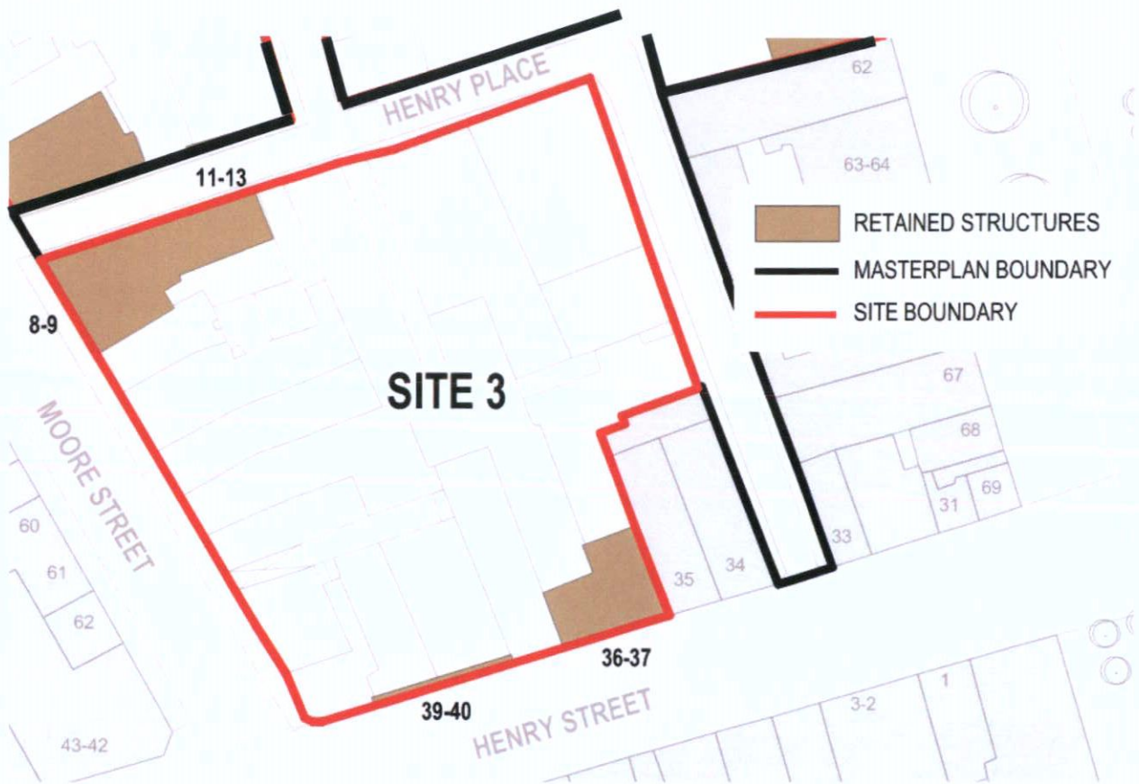
Figure 16 - Site 3 Retained Structures
