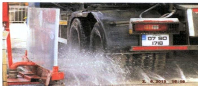
Figure 8 – Typical Wheel Washing Facility
