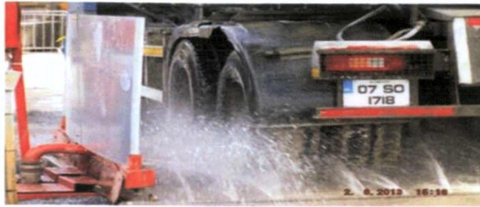
Figure 8 – Typical Wheel Washing Facility
