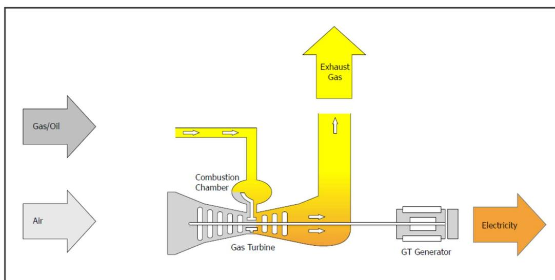
OCGT units are advantageous due to their operational flexibility and can be turned on quickly to provide peak load. The LEL Flexgen Castlelost reserve generator is designed to get to full load in less than 10 minutes. OCGTs exhaust residual heat to atmosphere at a temperature of approximately 544°C, i.e., unlike combined cycle gas turbines (CCGTs) where exhausted heat is recycled to generate steam and ultimately additional electricity. The OCGT units have a typical energy efficiency of 38-41%.
