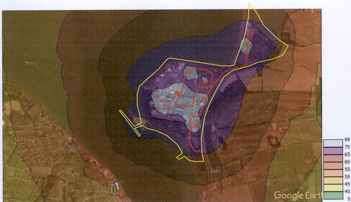
Figure 14.14 Predicted cumulative contours from likely worst case noise scenario during enabling works construction/demolition and Gouldings construction. N1
