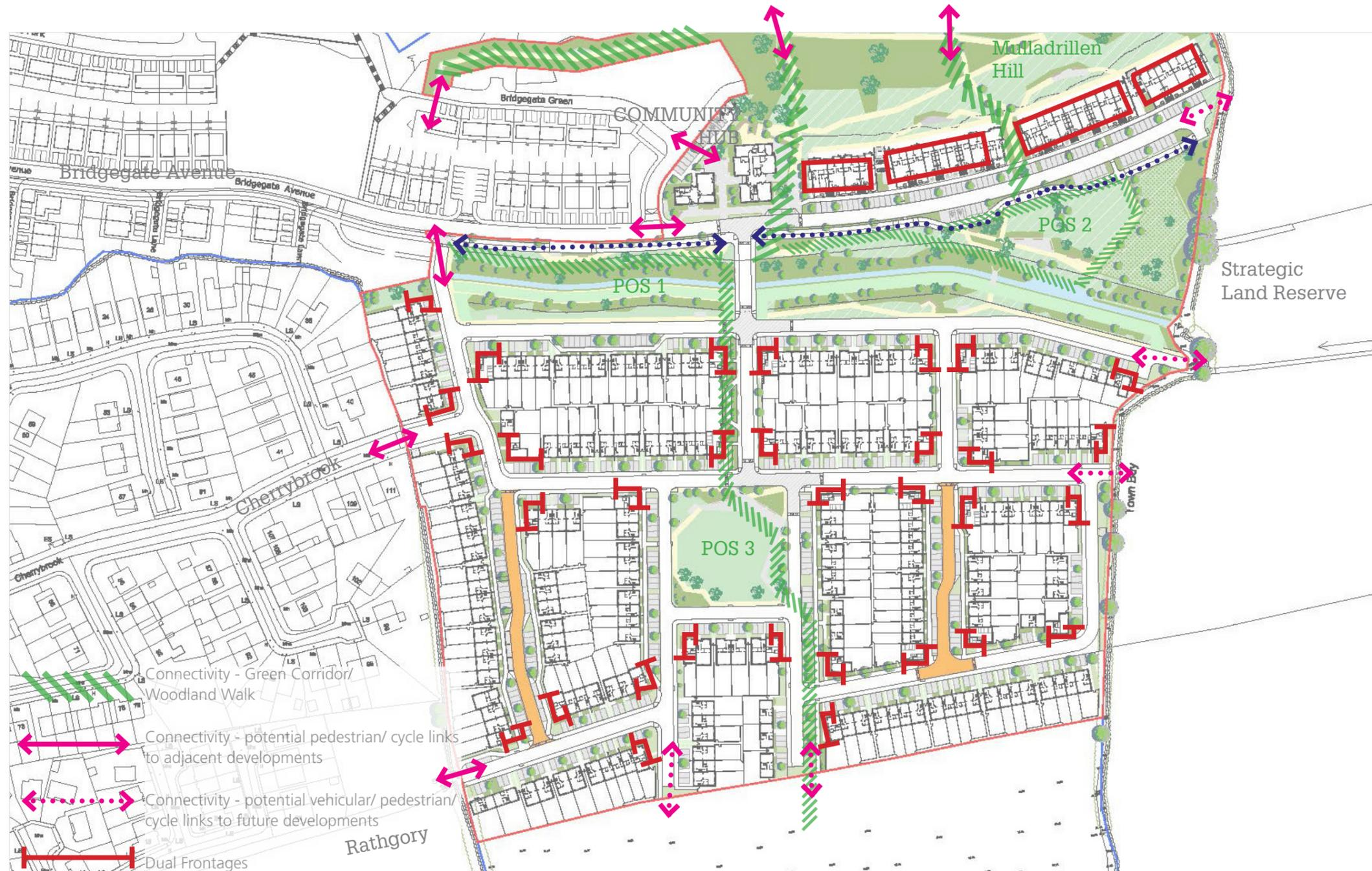
The proposed layout has been carefully arranged to create a permeable interconnected series of routes that extend/ integrate with adjacent established communities to the west & potential future developments to the south & east that are easy and logical to navigate around.
