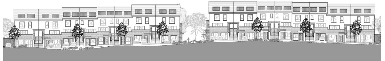
▲ Three Storey stepped facades with selected brick to the lower bays, and lower gable returns. Elevation & street frontage is further animated with patio and terraces to ground & first floor levels.
