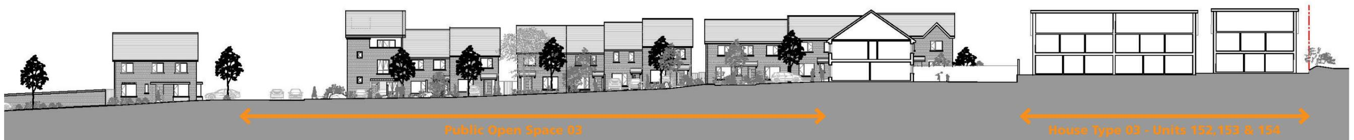
▲ Part section CC - 2 storey terrace houses with Duplex corner unit overlooking POS 03. No overlooking from House Type 03 at first floor to the rear of their properties. Note, rear access is provided for all units to back gardens for private access & bin storage
