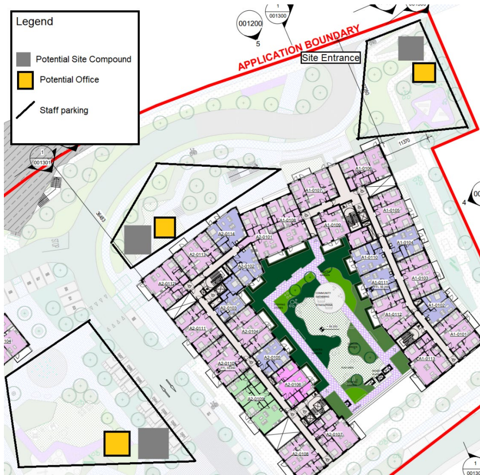
Figure 3.1 Site construction compound location
