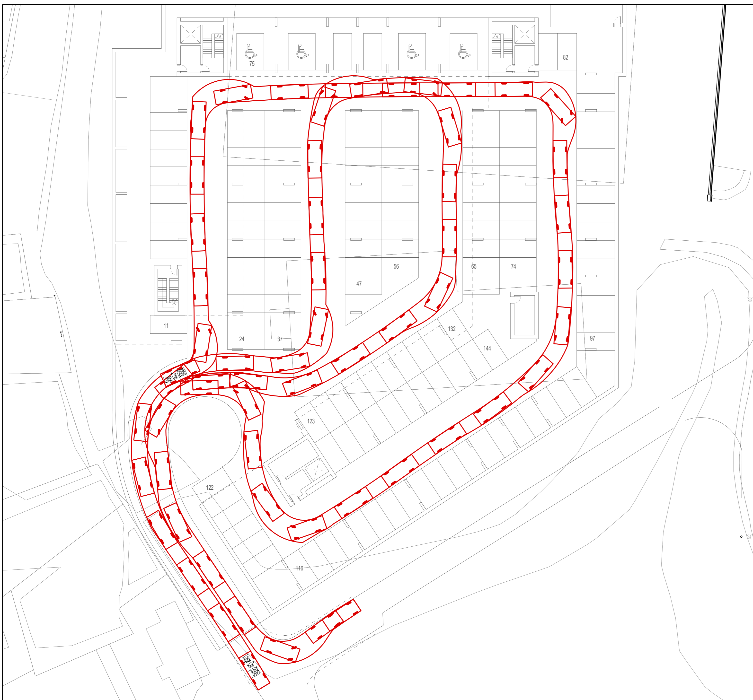
LARGE CAR BASEMENT ENTRY/EXIT
