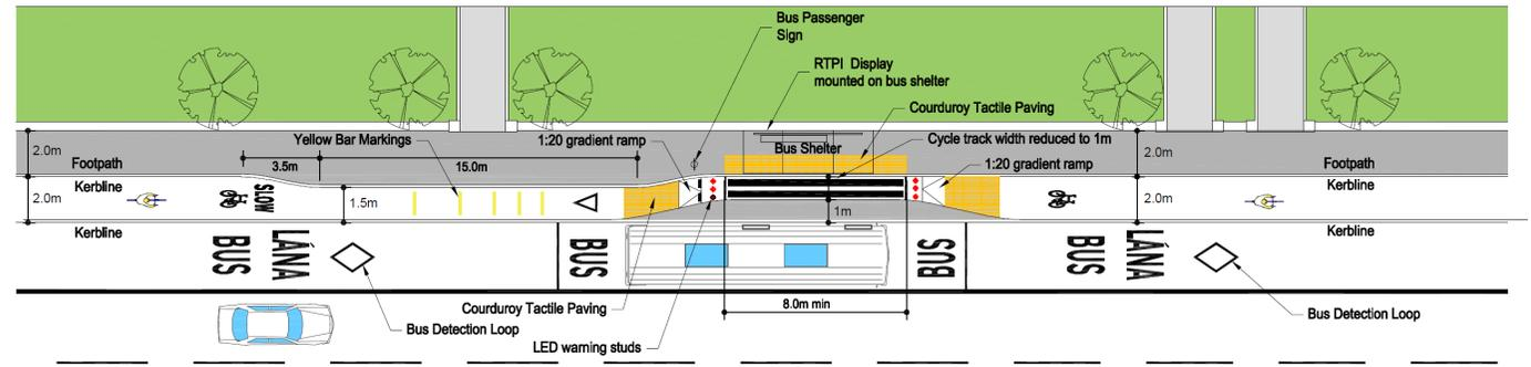
Figure 35: Shared Bus Stop Landing Zone Arrangement
