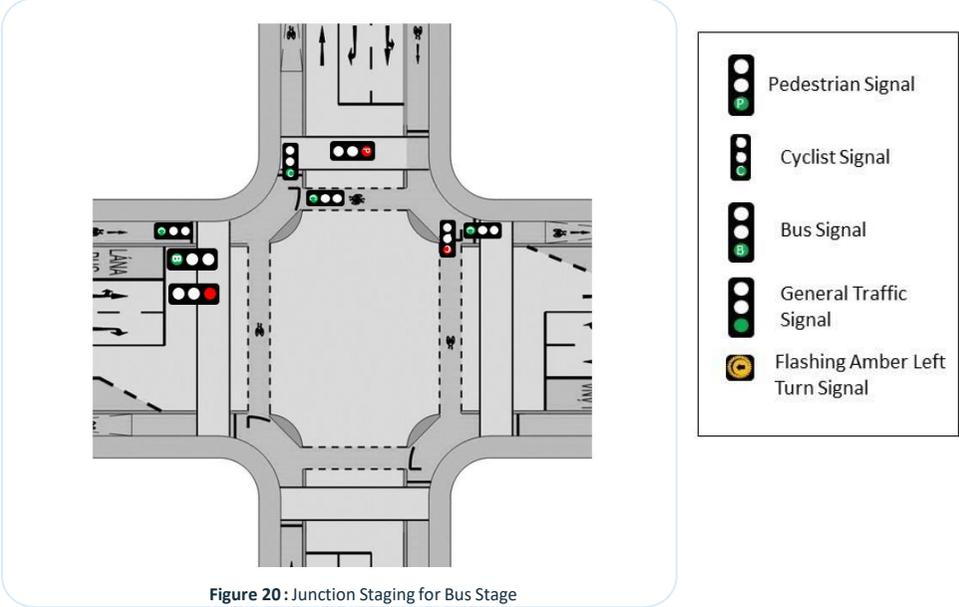
Figure 20: Junction Staging for Bus Stage
