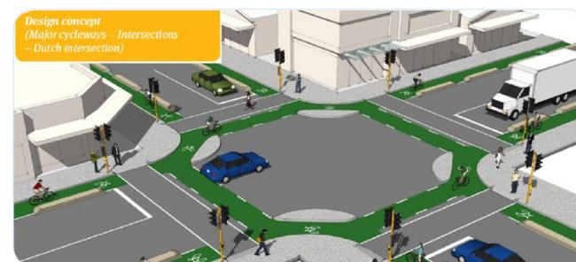
Figure 16: Key Infrastructure Elements of Protected Junction
