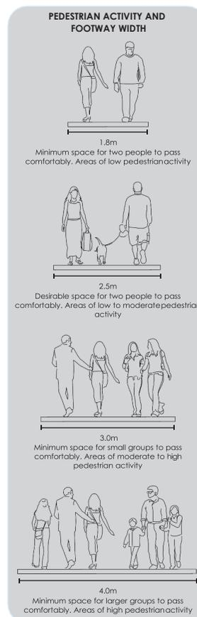
**Figure 10:** Extract from DMURS indicating appropriate footpath widths
