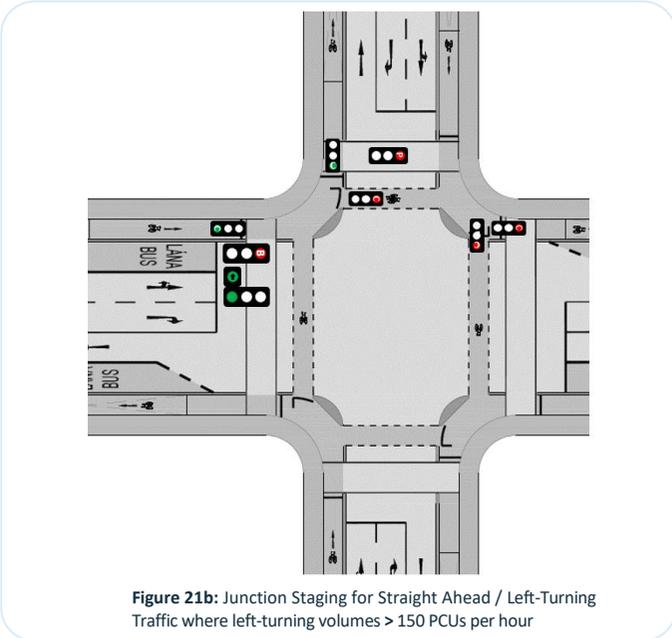
Figure 21b: Junction Staging for Straight Ahead / Left-Turning Traffic where left-turning volumes > 150 PCUs per hour
