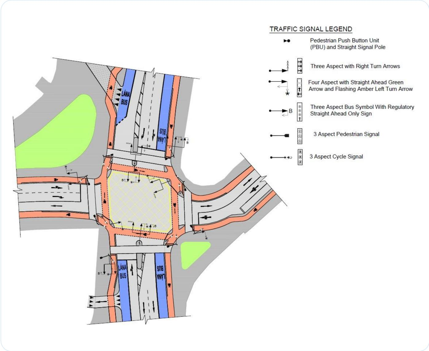
Figure 22: Indicative Traffic Signal and Phasing Layout
