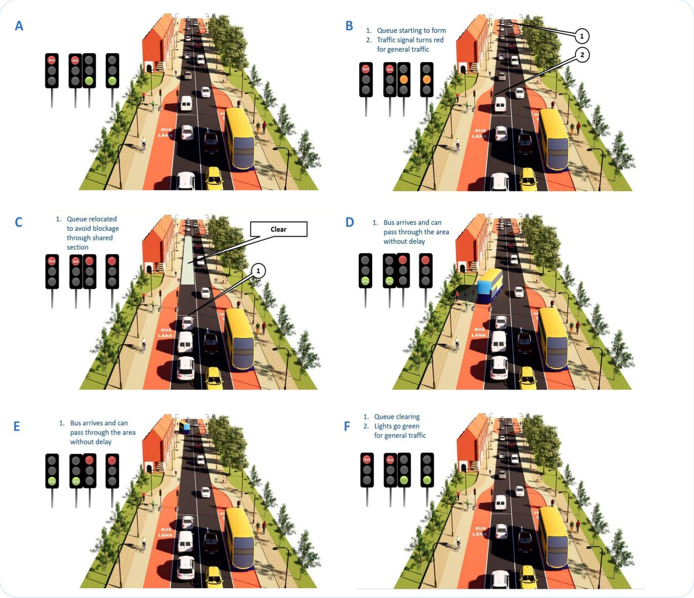
Figure 33: Bus Priority Traffic Signal Schematic Operation
