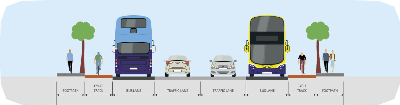
Figure 1: Optimum CBC Cross-Section
