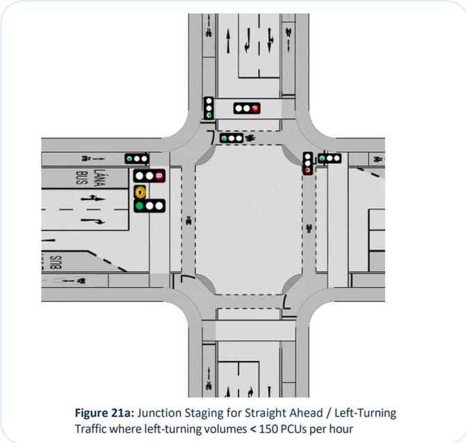
Figure 21a: Junction Staging for Straight Ahead / Left-Turning Traffic where left-turning volumes < 150 PCUs per hour
