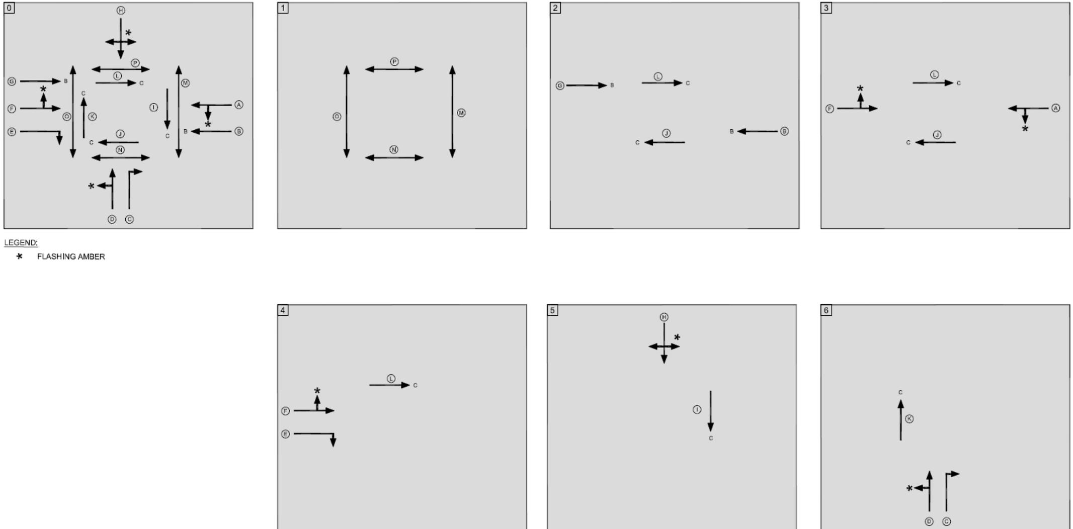
Figure 23: Indicative Junction Phasing and Staging Diagram
