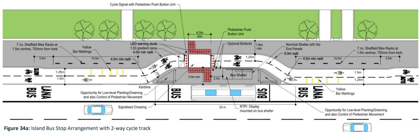
Figure 34a: Island Bus Stop Arrangement with 2-way cycle track
