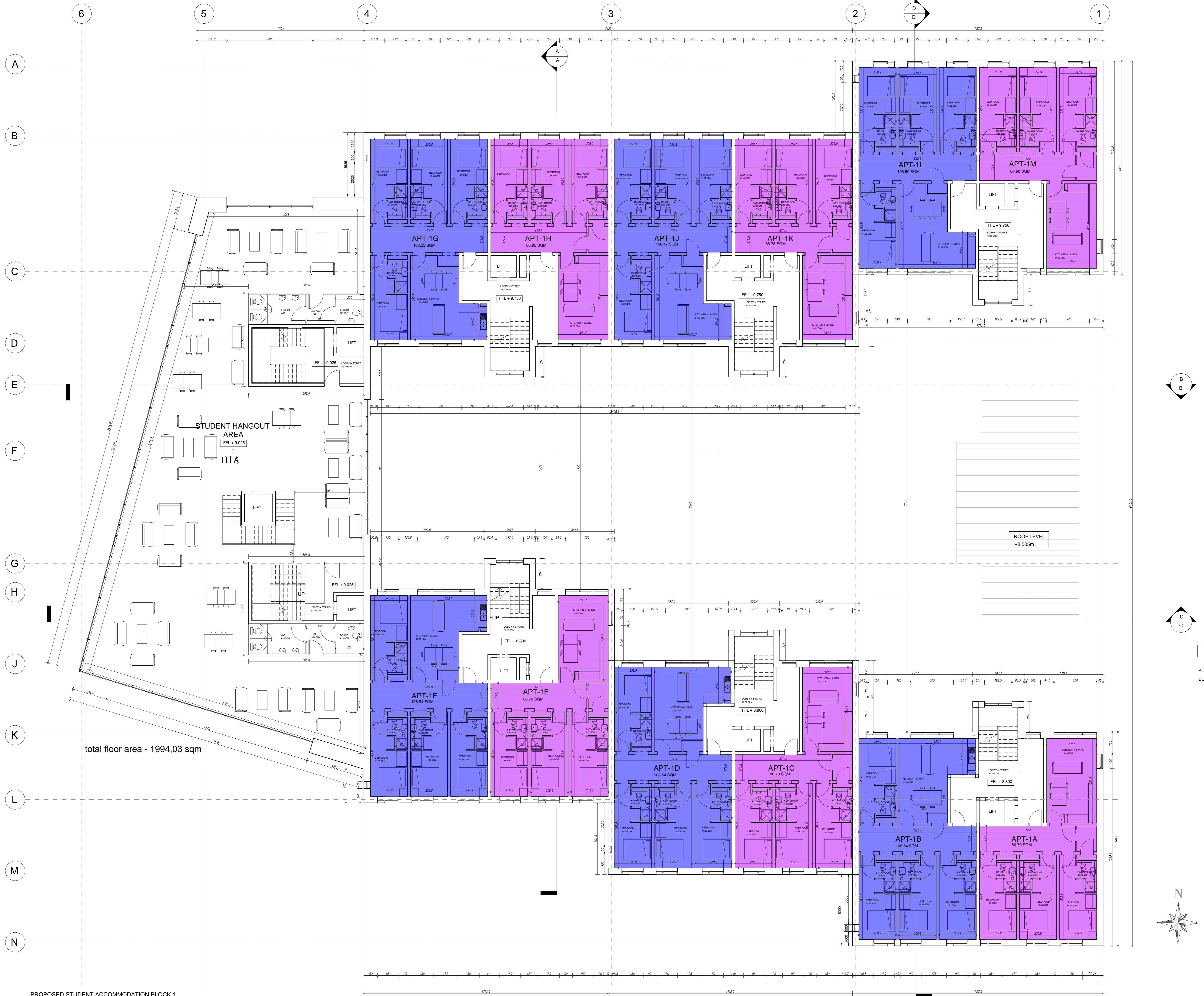
PROPOSED STUDENT ACCOMMODATION BLOCK 1 FIRST FLOOR PLAN 1:100
