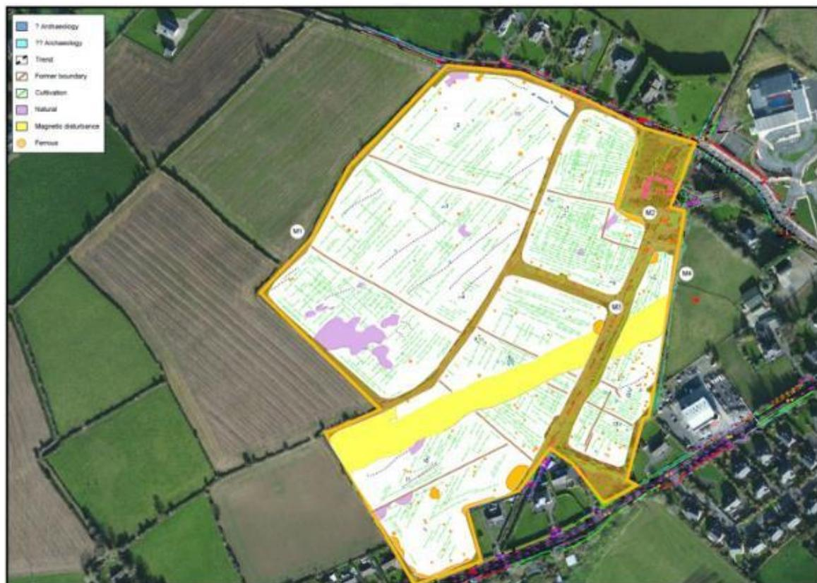
Figure 6 Geophysical Survey Interpretation Drawing.
