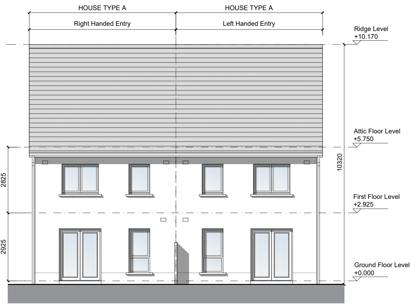
REAR ELEVATION (Terrace Type A-A) Scale 1:100
