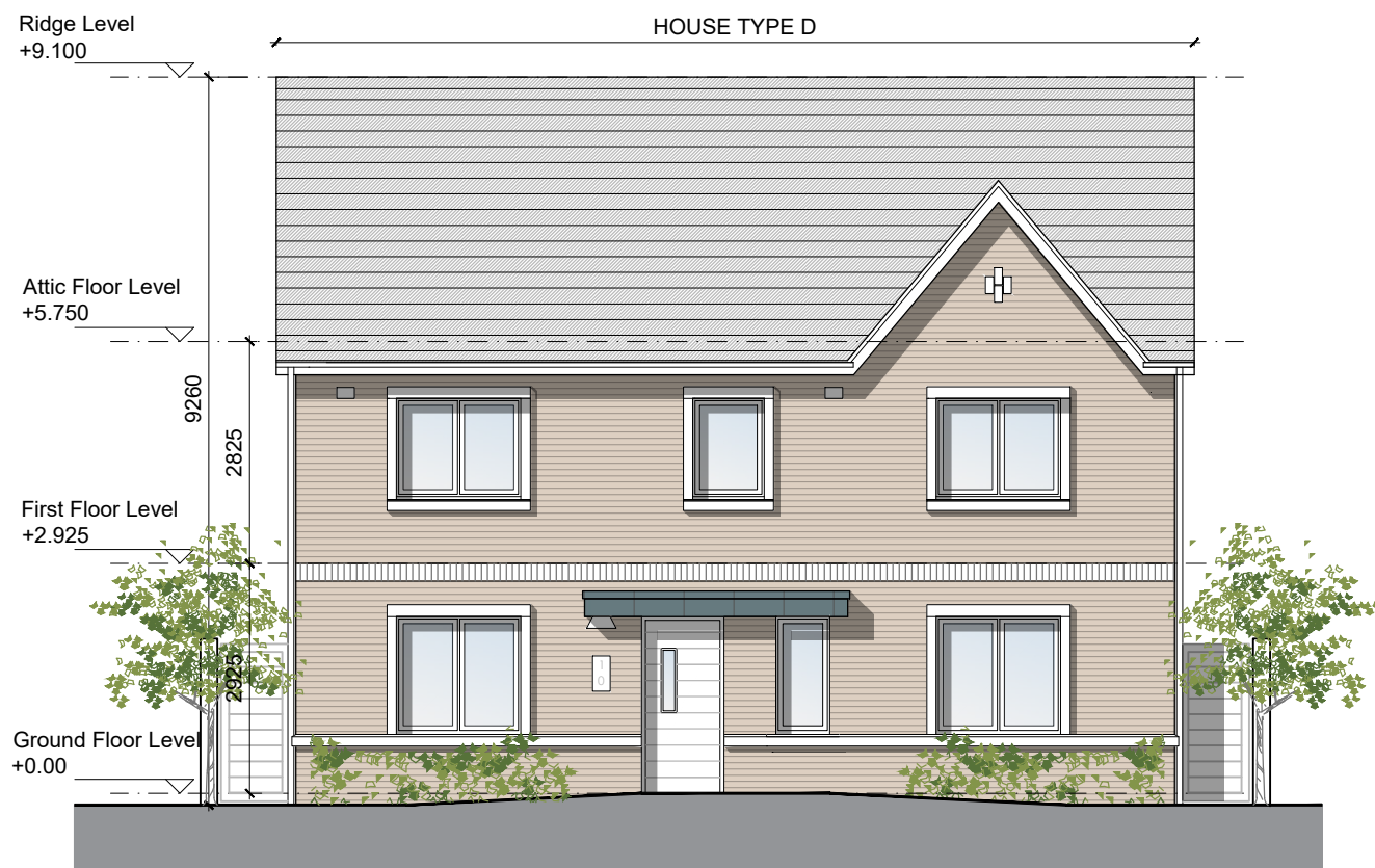
FRONT ELEVATION (Detached Type D) Scale 1:100
