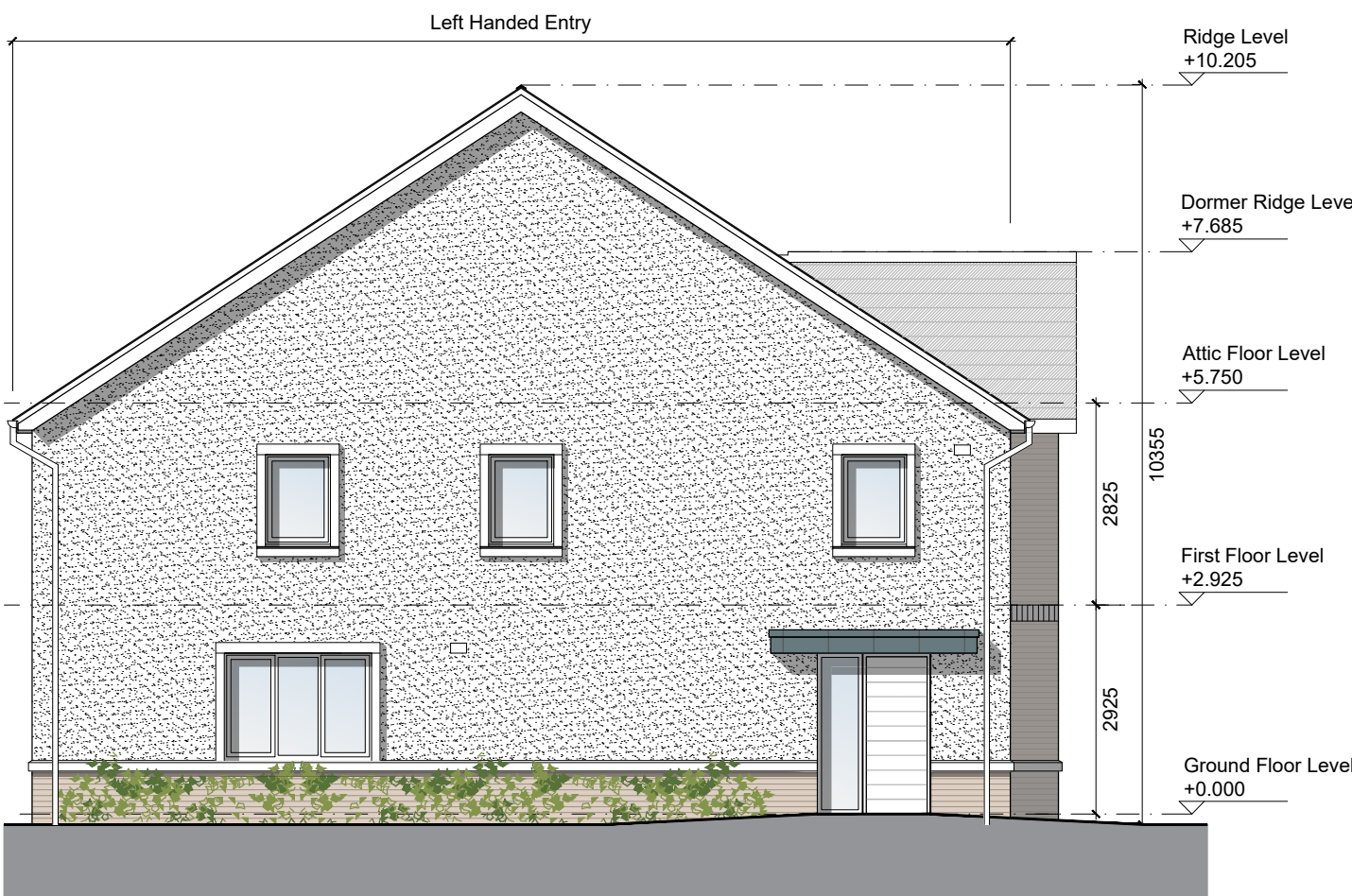
SIDE ELEVATION (Semi Detached Type F1) Scale 1:100
