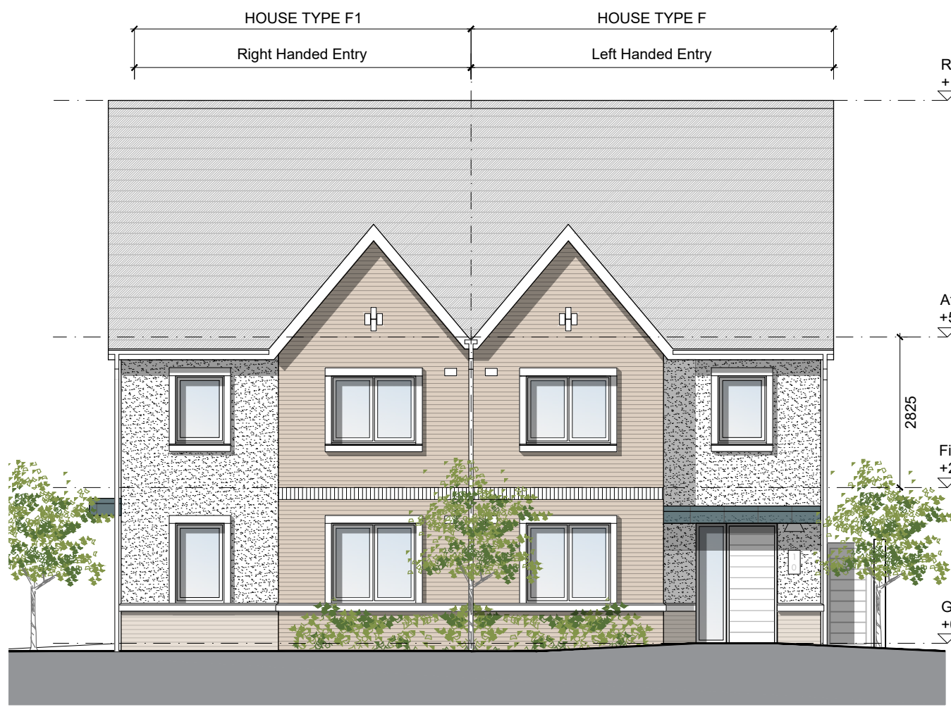
FRONT ELEVATION (Semi Detached Type F1-F) Scale 1:100
