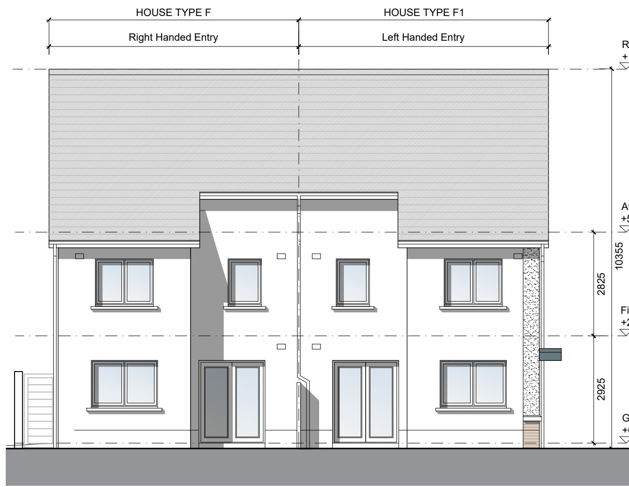
REAR ELEVATION (Semi Detached Type F-F1) Scale 1:100
