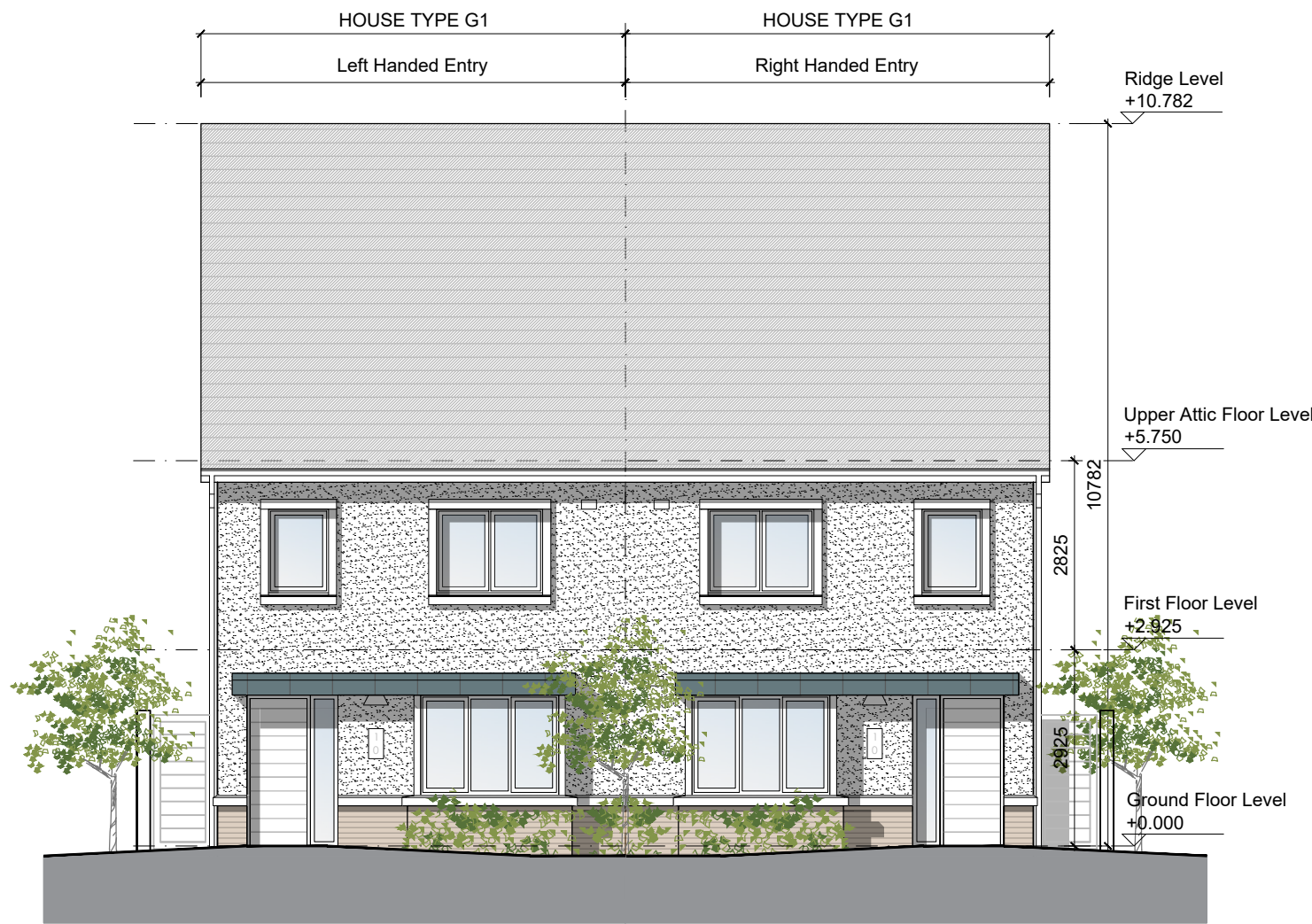
FRONT ELEVATION (Semi Detached Type G1-G1) Scale 1:100
