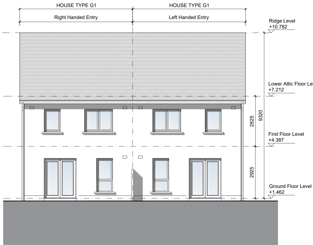
REAR ELEVATION (Semi Detached Type G1-G1) Scale 1:100
