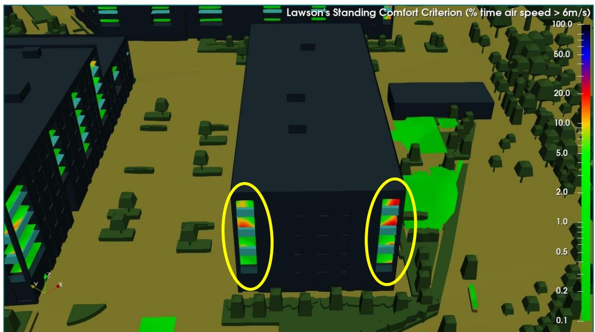
Figure 8: Standing Comfort Criterion: Balconies of block D
