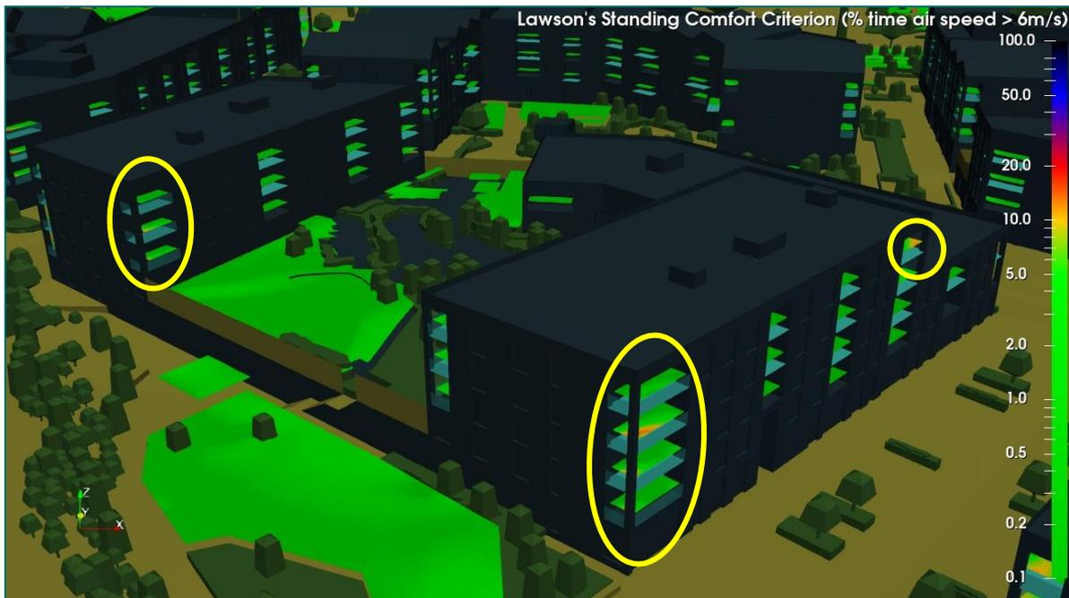
Figure 10: Standing Comfort Criterion: Balconies of block E
